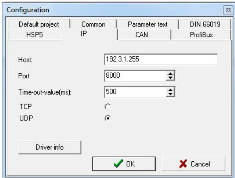
If configured that way COMBIVIS addresses the devices via the IP address 192.10.1.x, where x corresponds to the configured node address. The used node address by COMBIVIS for addressing the unit must agree with the adjusted value of parameter Din66019SlvAddr. Please observe from software V2.5 of the F5 PROFINET operator the Din66019SlvAddr is linked to the Pnet\_IPAddress by way that Din66019SlvAddr = last digit of Pnet\_IPAddress.
