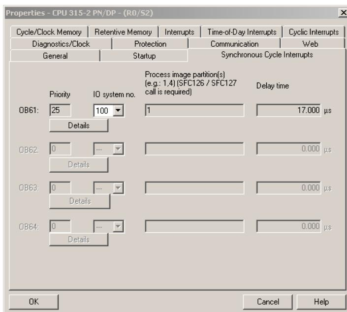
The detail adjustments must be done via the button 'details' of the selected OB.
