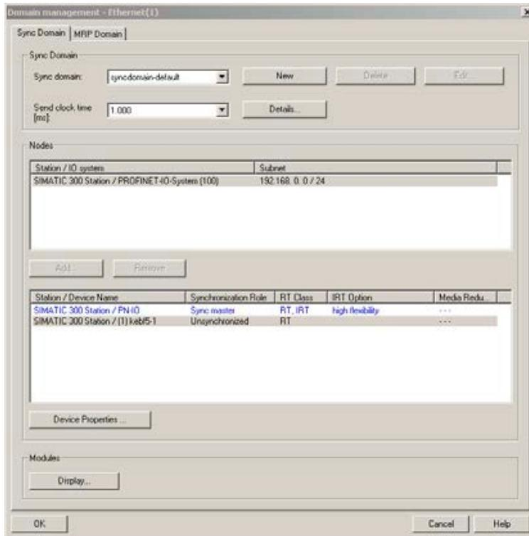
It makes sense to set the transmit clocking to 2ms, because this corresponds to the minimum setting of the KEB F5 PROFINET slave. Furthermore the KEB slave is selected here (click on 'kebf5-1') and configured as follows via clicking the button 'unit characteristics':
