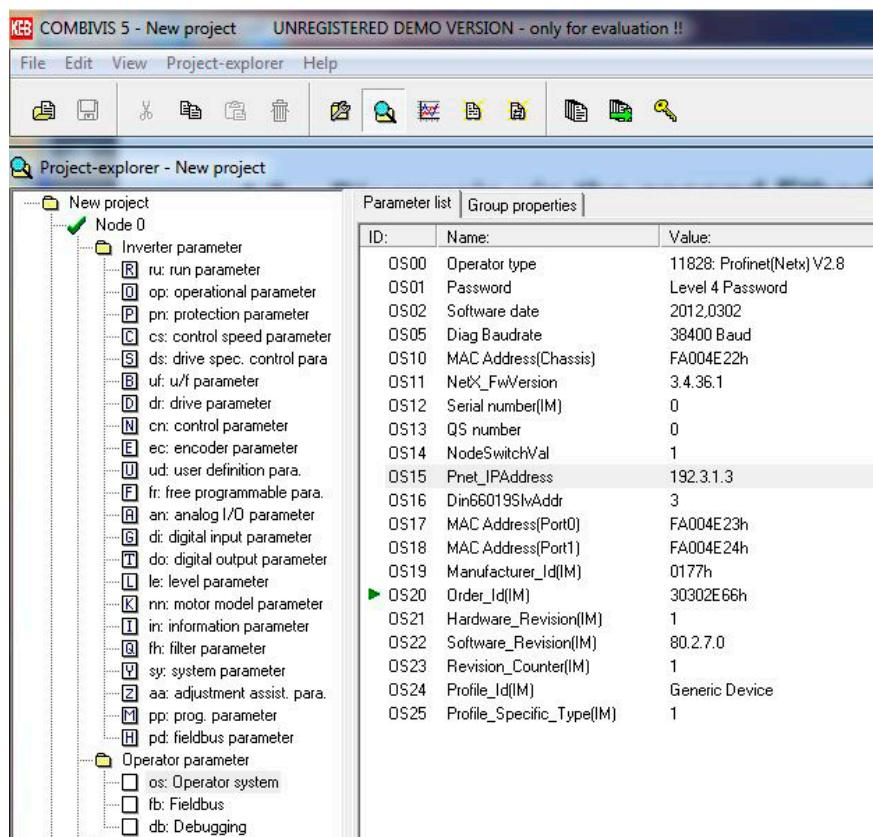
By setting the last digit of the host IP address to value = 255 in the IP configuration of COMBIVIS one ensures that COMBIVIS can address several connected IP devices whose IP address is in the range 192.10.1.x.
