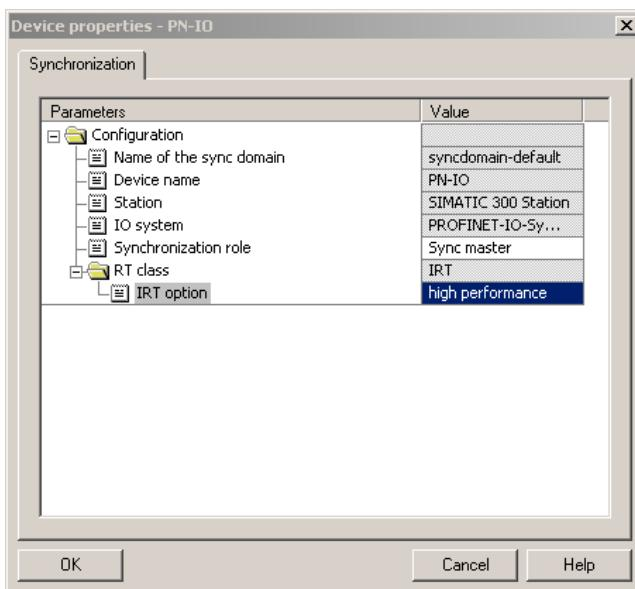
Then in the right part of the HW Config window of PROFINET-IO → additional field instruments → ....the KEB F5 PROFINET operator selected and appended with the mouse to the PROFINET System in the left pane. It is important that the PROFIDRIVE\_PAP module is placed into slot 3:
