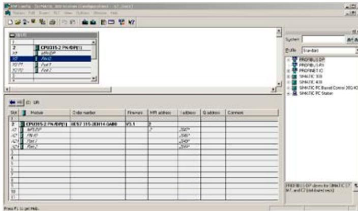
If the synchronous communication (PROFINET IO-IRT) shall be used, the PN-IO interface of the CPU can be configured by right-clicking on the PN-IO interface of the CPU and select object properties as a sync master:
