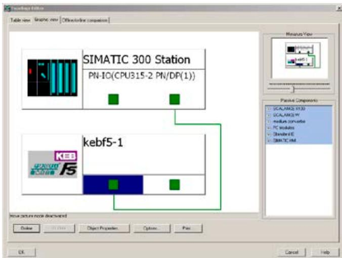
Then the KEB slave must be configured as sync slave via right-click to the PROFINET IO system and selection of PROFINET domain management.
