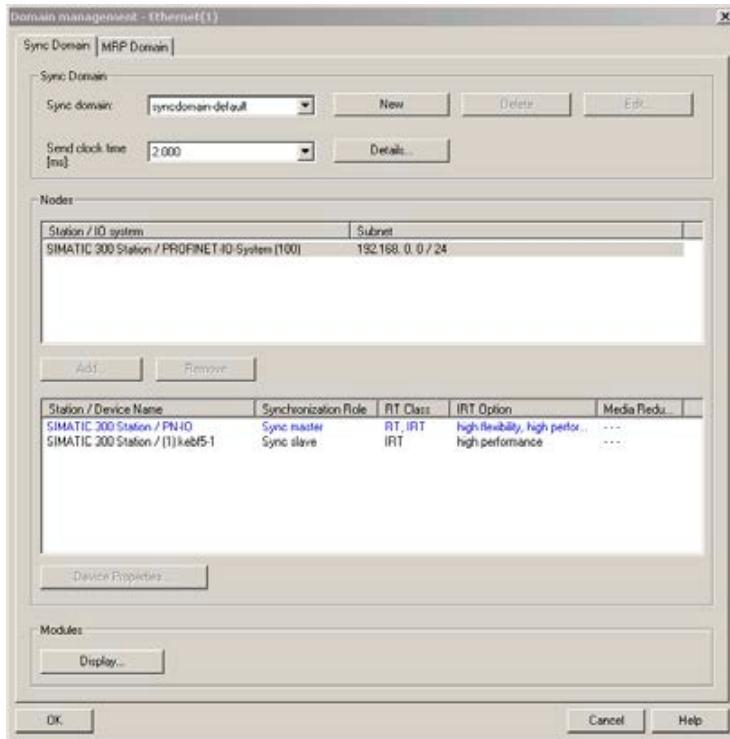
The Siemens S7 plc provides synchronous alarms for synchronous communication. The exchange of synchronous, cyclic data is programmed in this alarm modules. The OB61 is activated for it in the example. This is done by right click to the CPU and selection of ,object characteristics'. Page ,synchronous alarm' is selected in the opening window.
