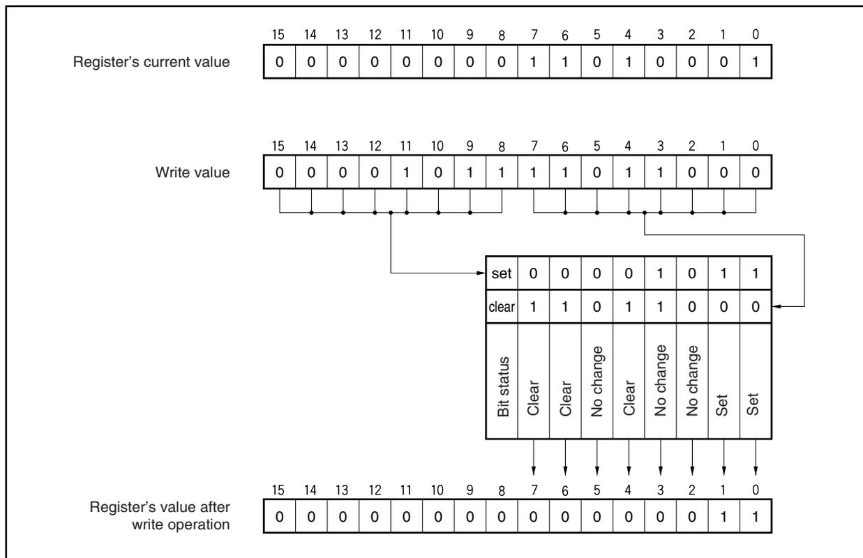
Figure 19-26. Bit Status After Bit Setting/Clearing Operations
