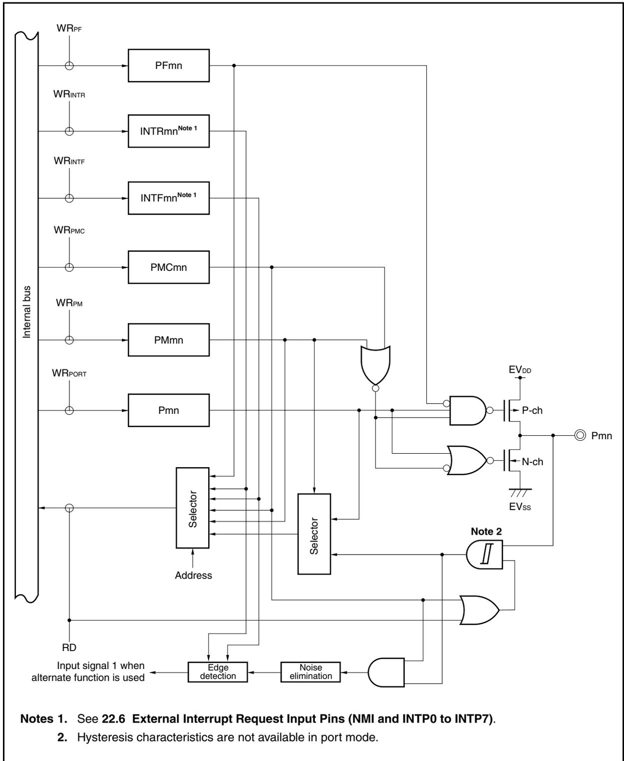
Figure 4-17. Block Diagram of Type N-1
