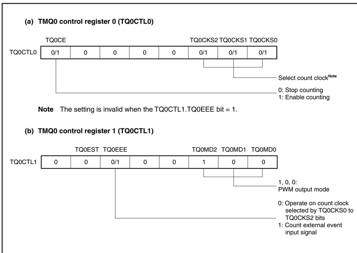
Figure 8-30. Setting of Registers in PWM Output Mode (2/3)
