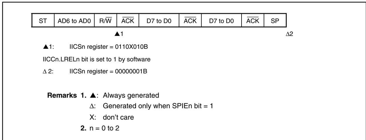
**(3) When arbitration loss occurs during data transfer****<1> When IICSn.WTIMn bit = 0**
