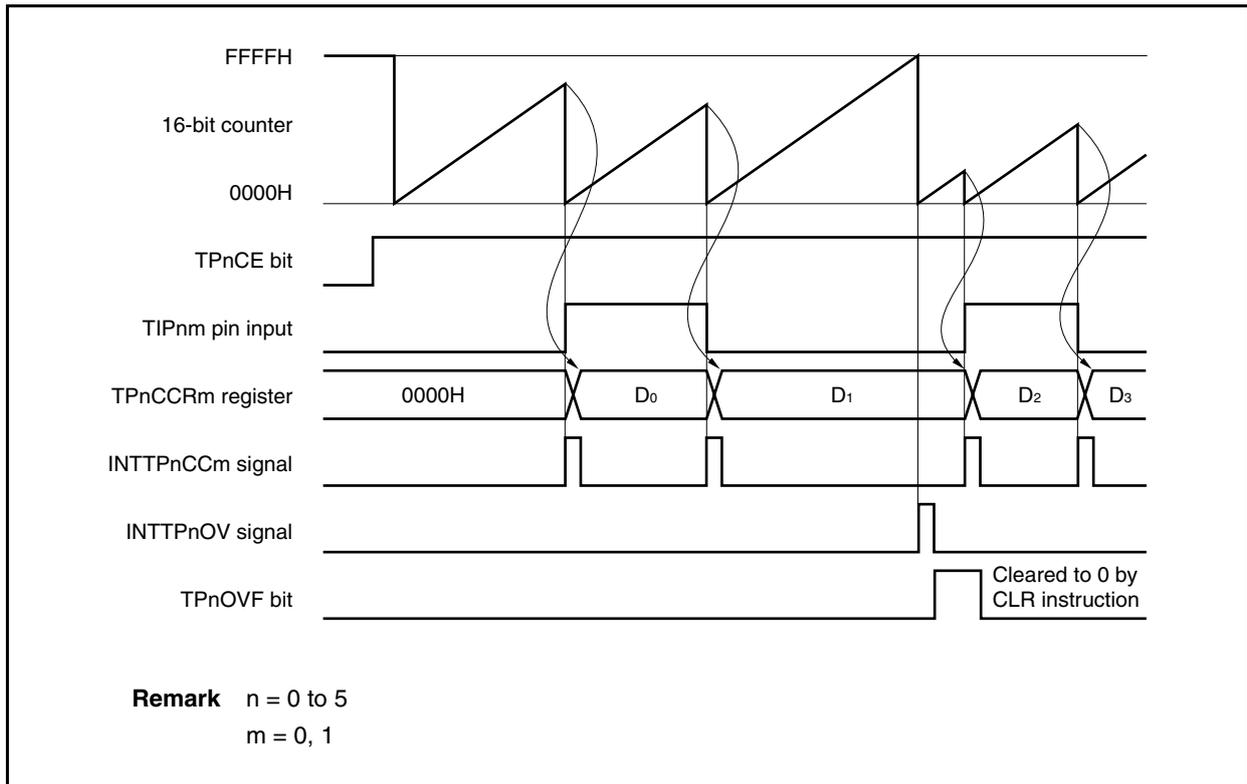
When the TPnCE bit is set to 1, the 16-bit counter starts counting. When the valid edge input to the TIPnm pin is later detected, the count value of the 16-bit counter is stored in the TPnCCRm register, the 16-bit counter is cleared to 0000H, and a capture interrupt request signal (INTTPnCCm) is generated.
