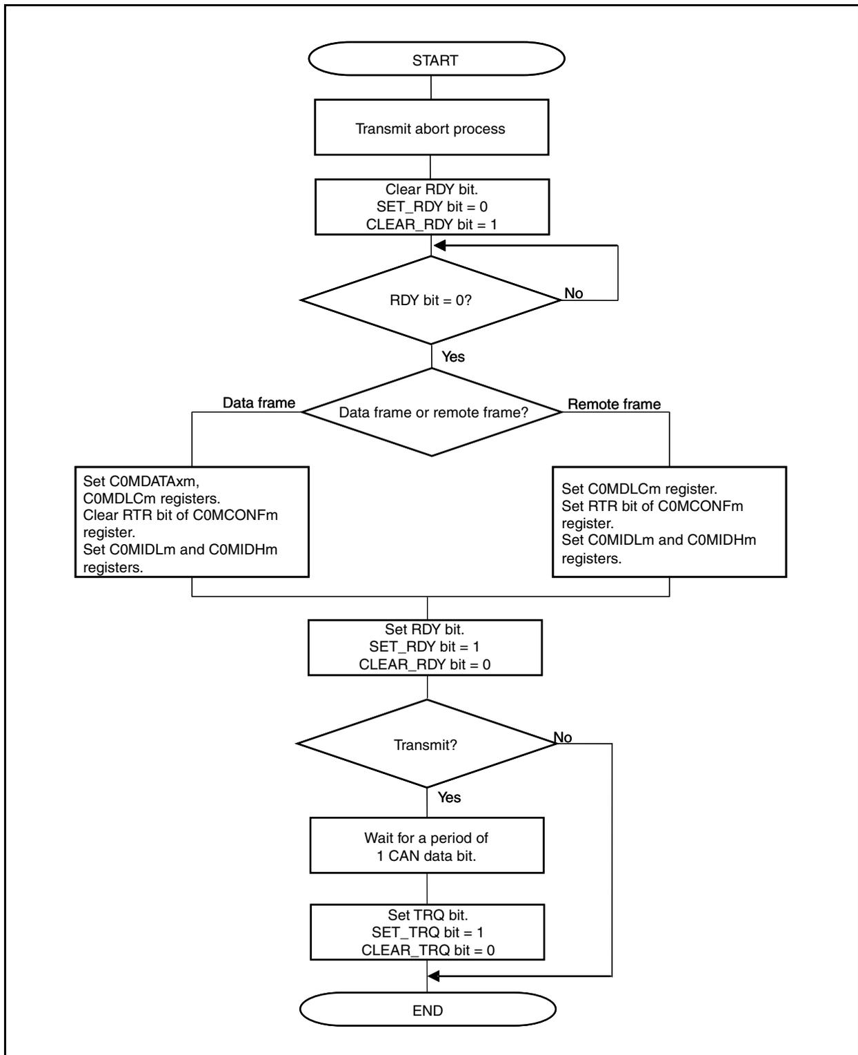
Figure 19-41 shows the processing for a transmit message buffer (COMCONFm.MT2 to COMCONFm.MT0 bits = 000B).
