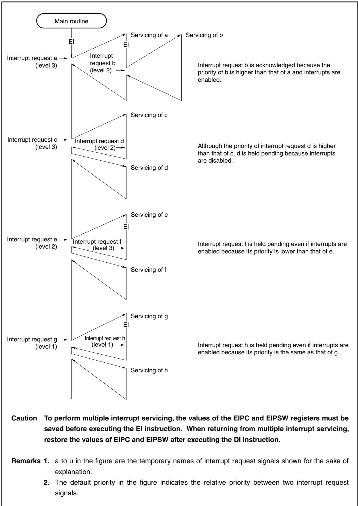
**Figure 22-7. Example of Processing in Which Another Interrupt Request Signal Is Issued While an Interrupt Is Being Serviced (2/2)**
