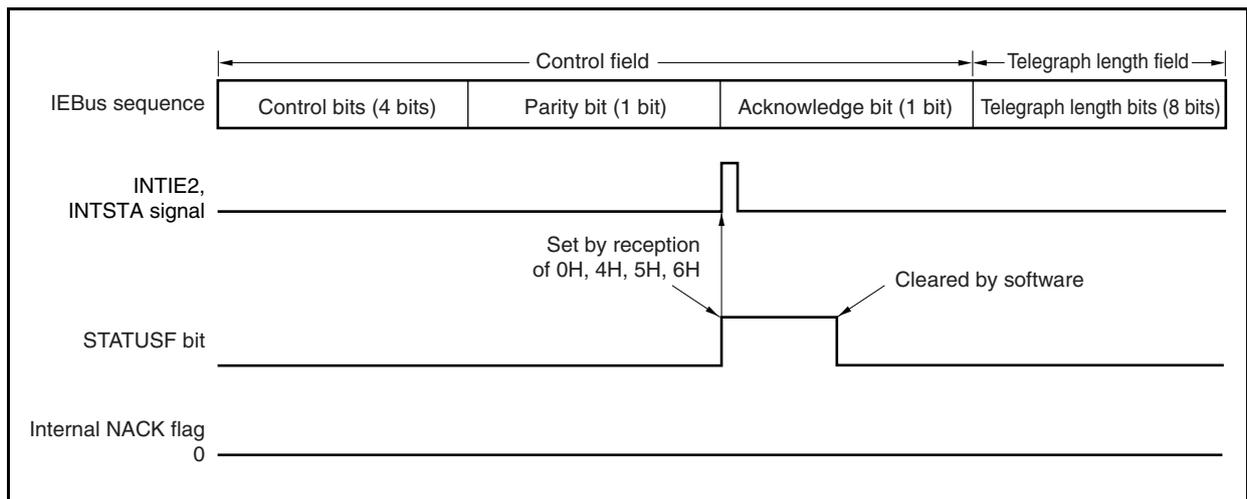
**Figure 18-17. Interrupt Request Signal Generation Timing (for (2) and (5))**
