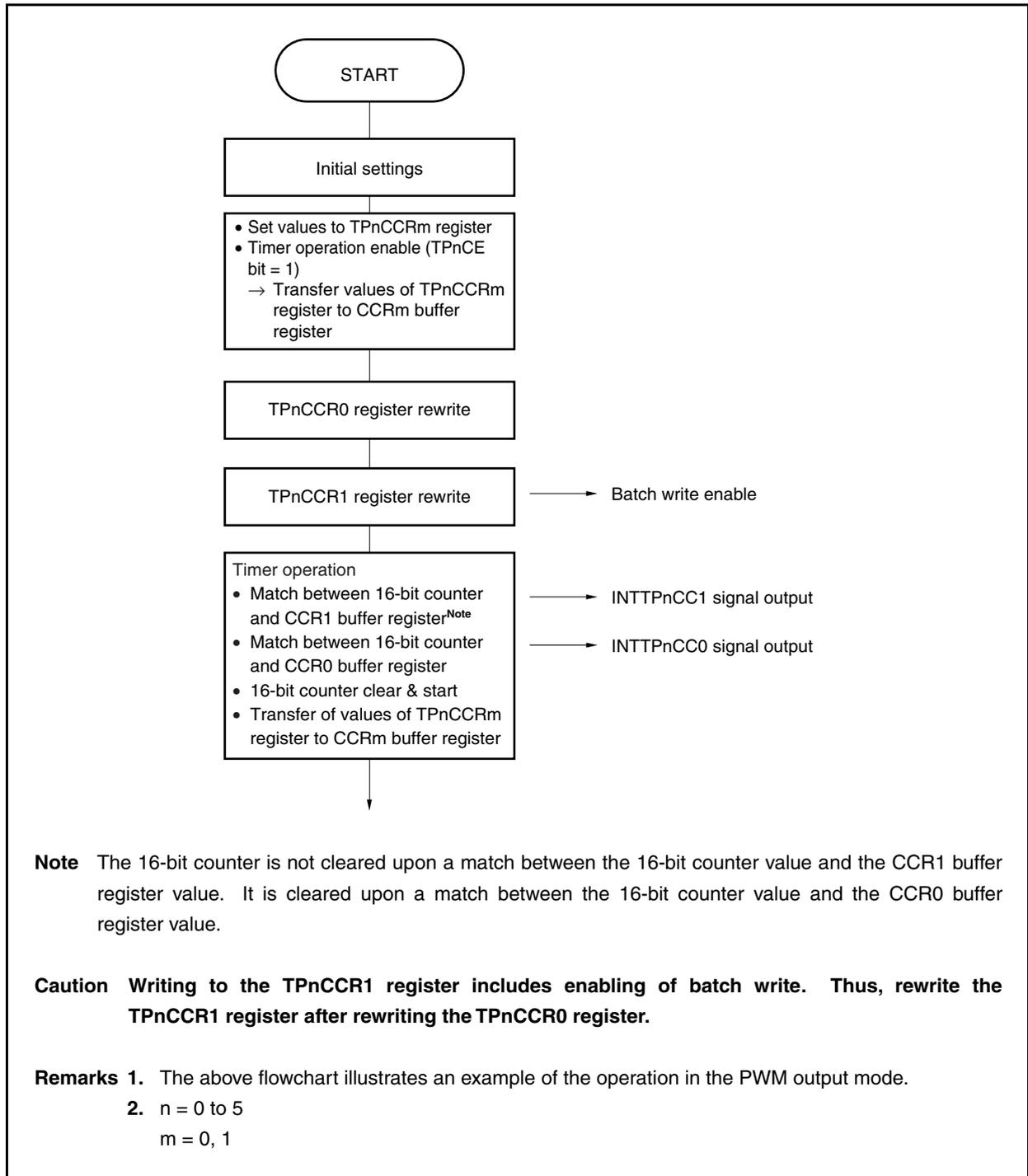
Figure 7-5. Timing of Batch Write
