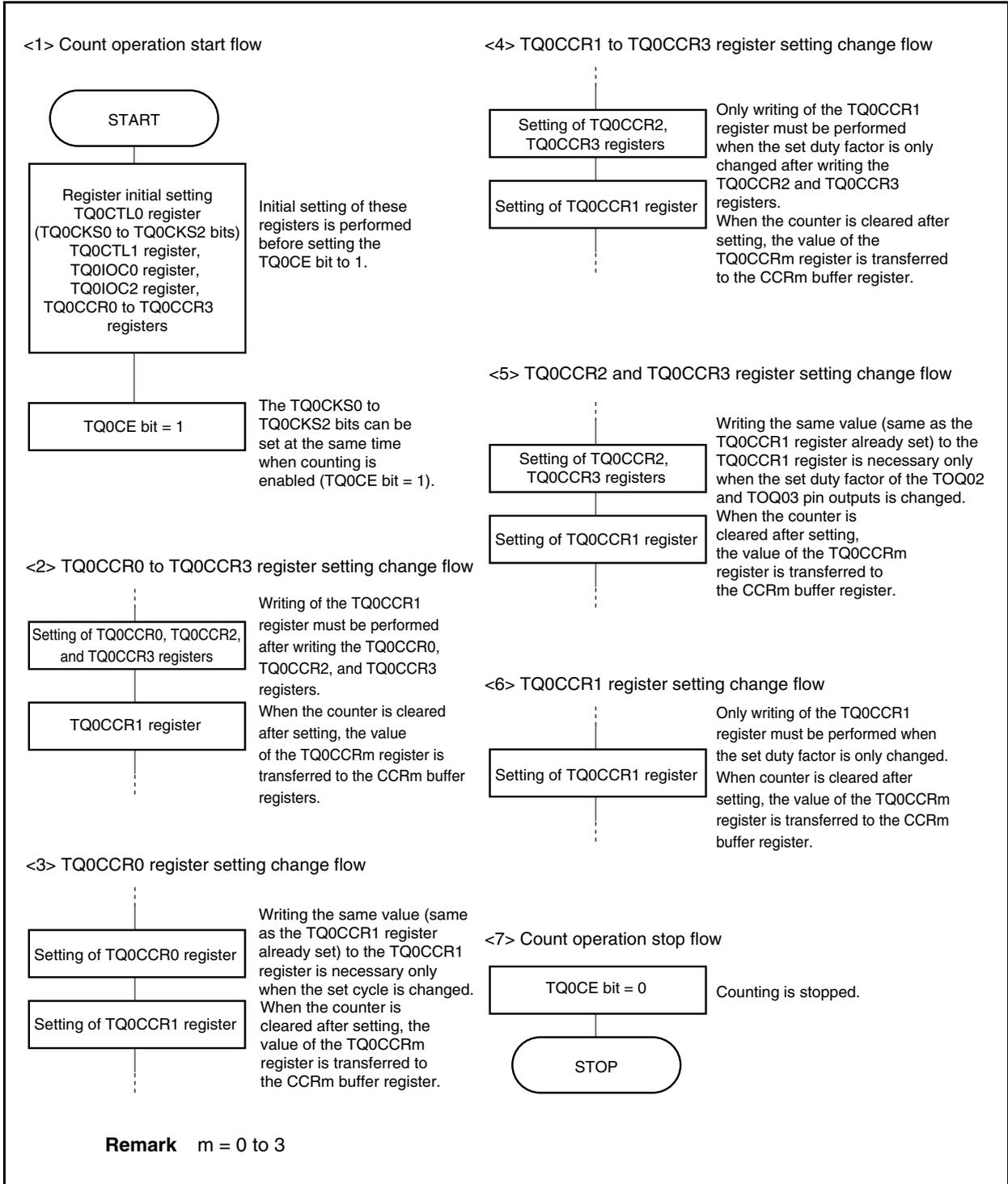
**(2) PWM output mode operation timing****(a) Changing pulse width during operation**
