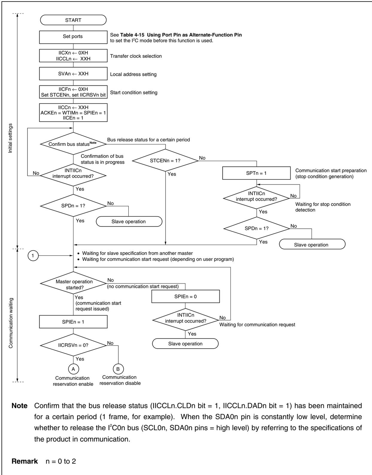
Figure 17-16. Master Operation in Multimaster System (2/3)
