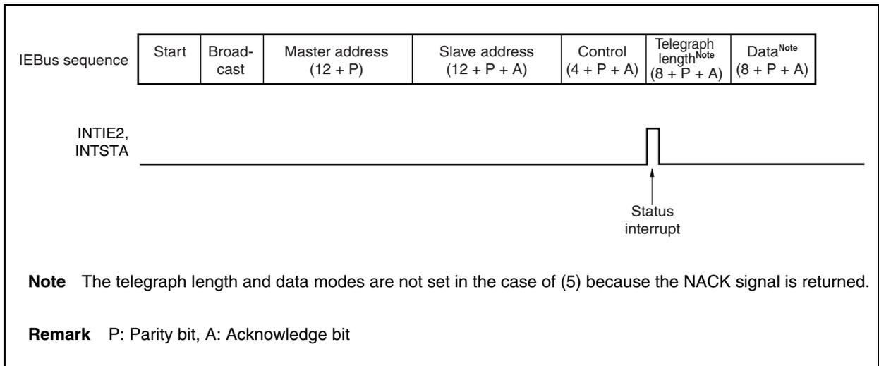
**Figure 18-19. Timing of INTIE2 and INTSTA Interrupt Request Signal Generation in Locked State (for (3))**
