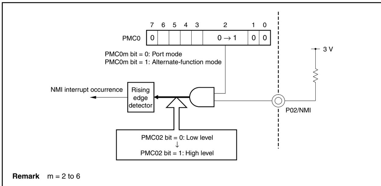
[Example 2] Switch from external pin (NMI) to general-purpose port (P02)
