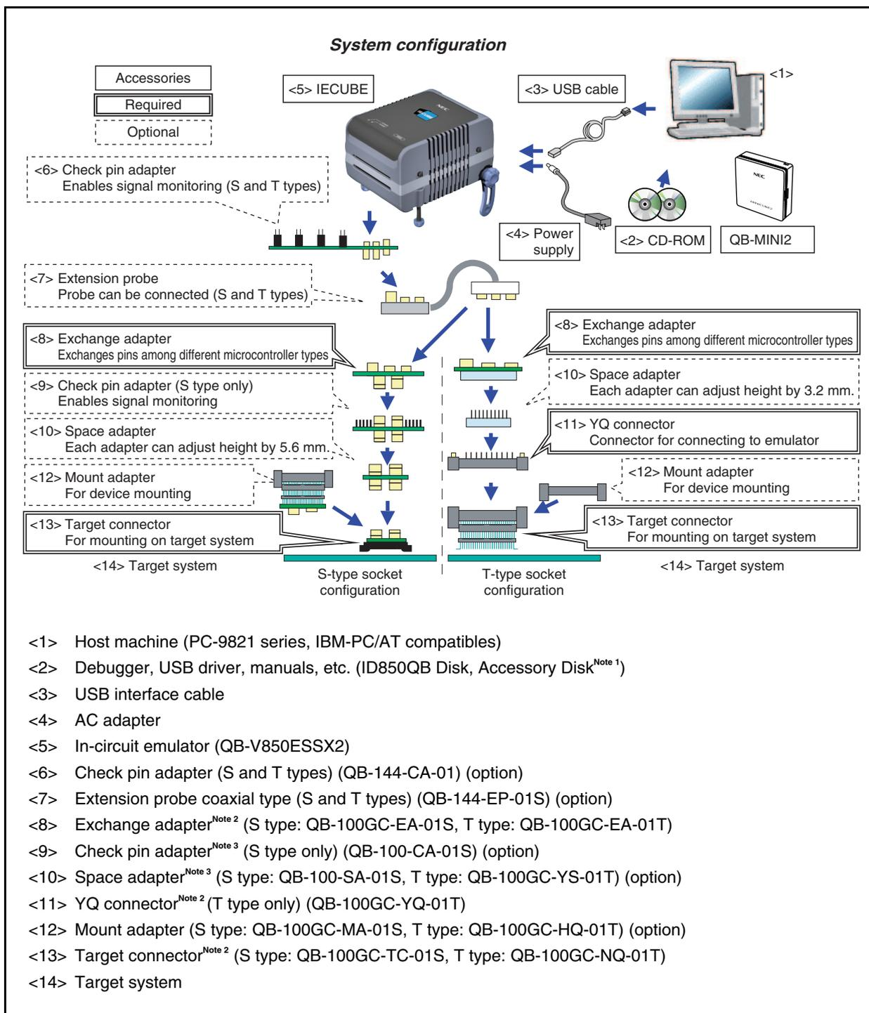
Figure A-3. System Configuration (QB-V850ESSX2 Used) (2/2)
