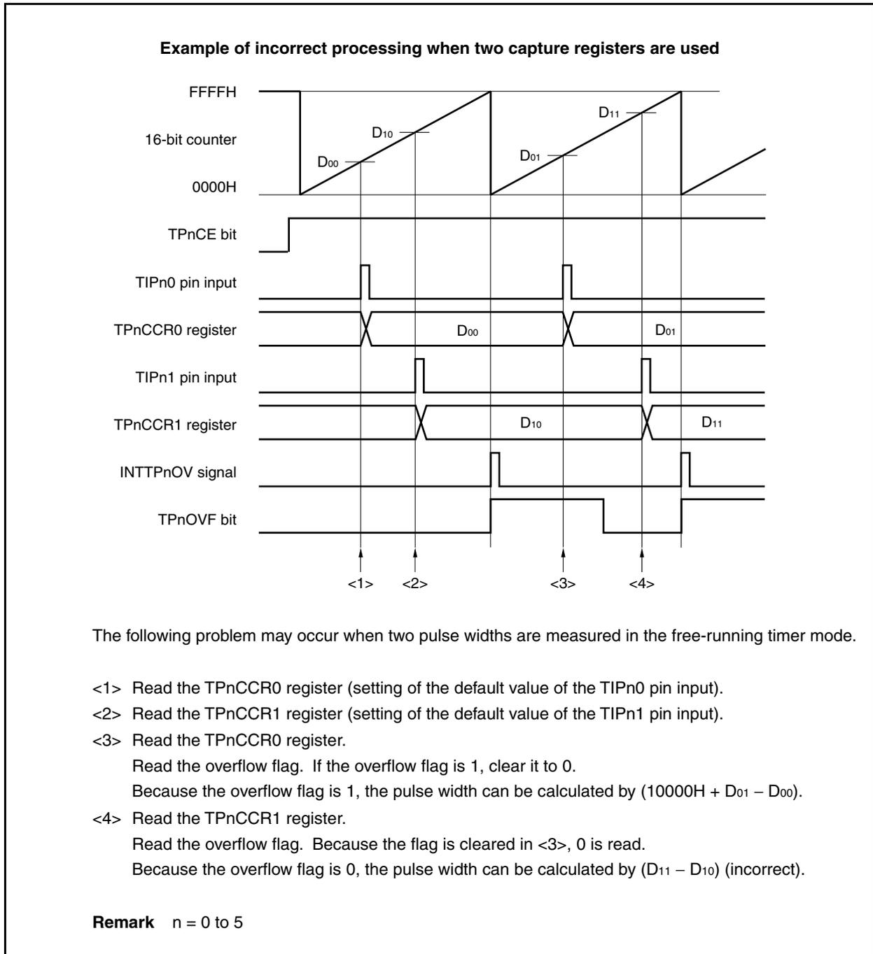
When two capture registers are used, and if the overflow flag is cleared to 0 by one capture register, the other capture register may not obtain the correct pulse width.
