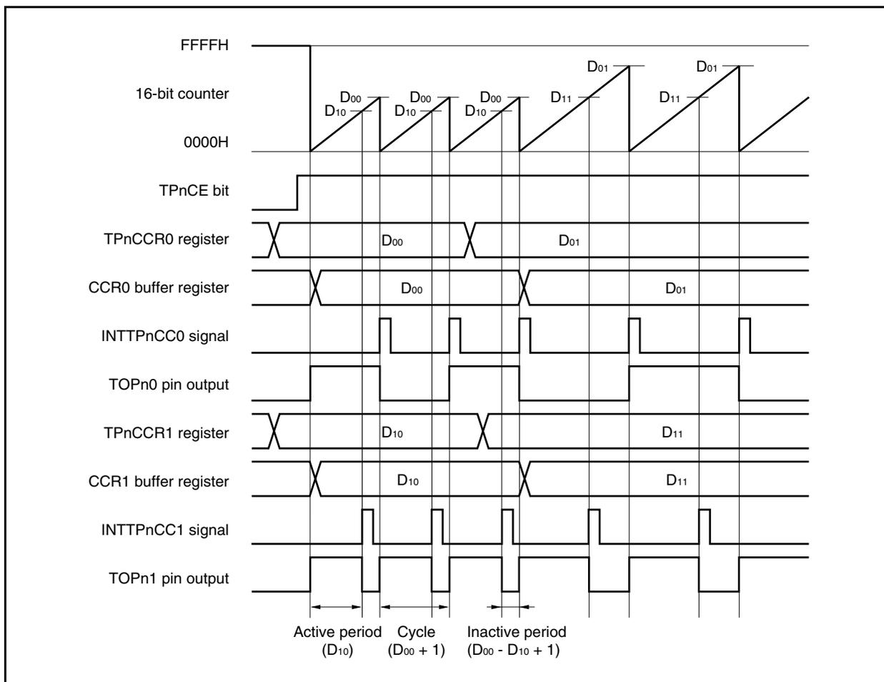
When the TPnCE bit is set to 1, the 16-bit counter is cleared from FFFFH to 0000H, starts counting, and outputs a PWM waveform from the TOPn1 pin.
