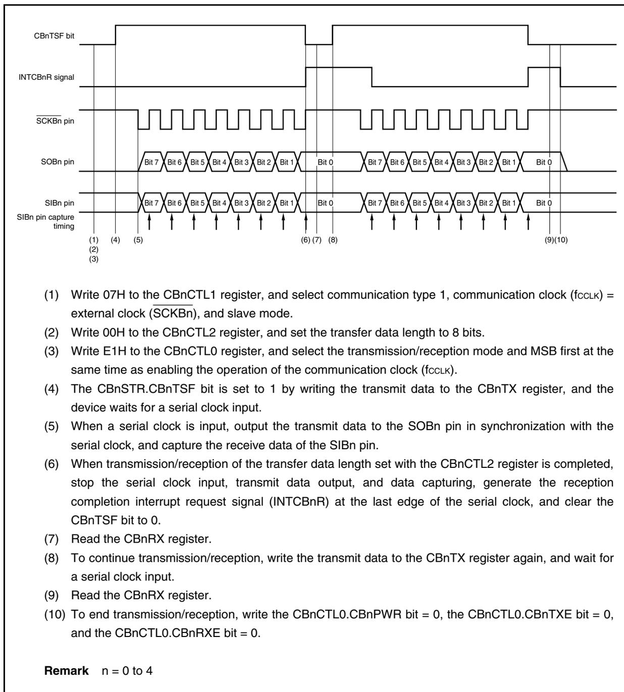
**16.6.7 Continuous transfer mode (master mode, transmission mode)**
