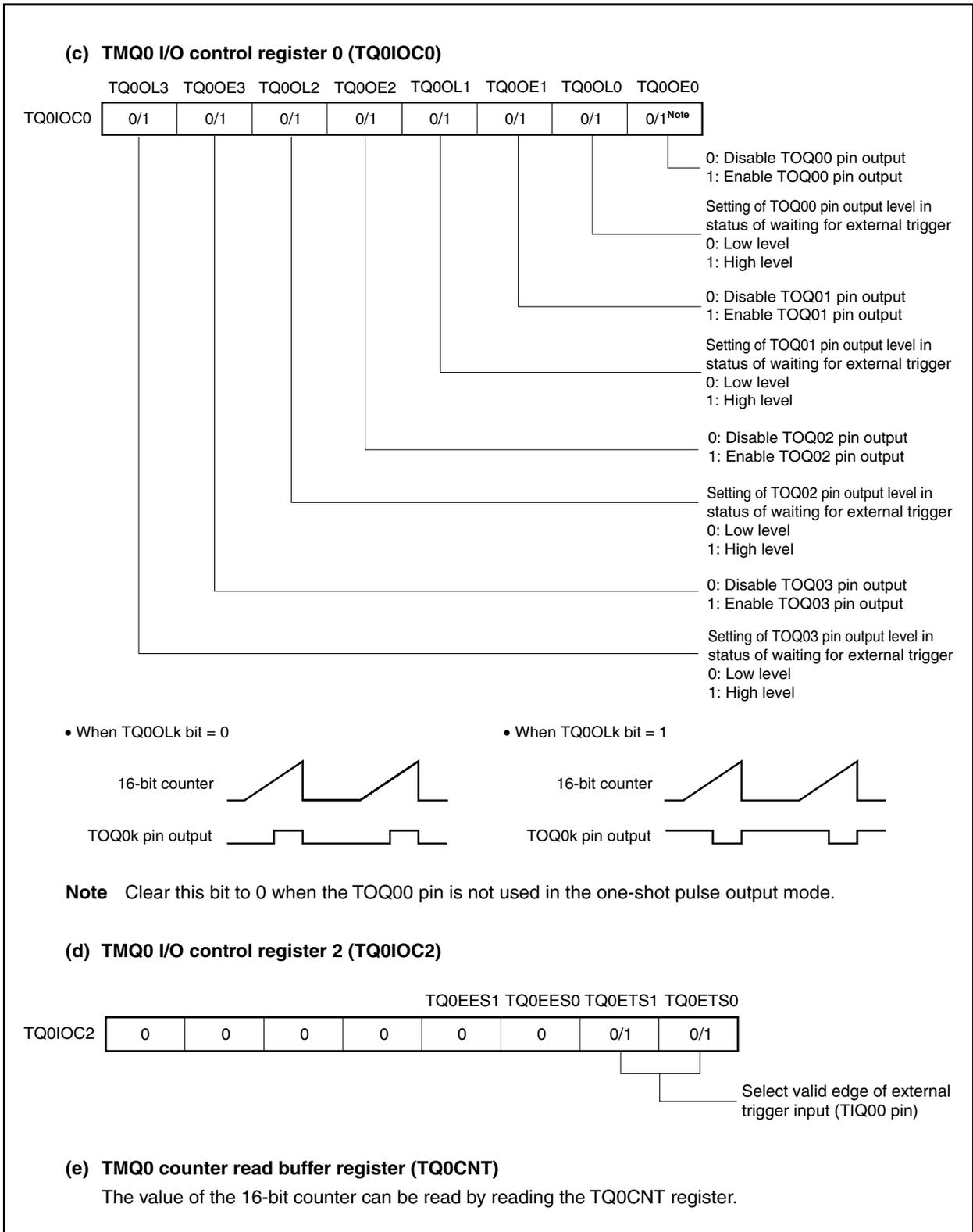
Figure 8-26. Register Setting in One-Shot Pulse Output Mode (3/3)
