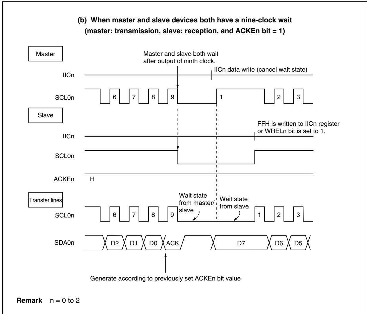
A wait state is automatically generated after generation of the start condition. A wait state is also automatically generated depending on the setting of the IICn.WTIMn bit.
