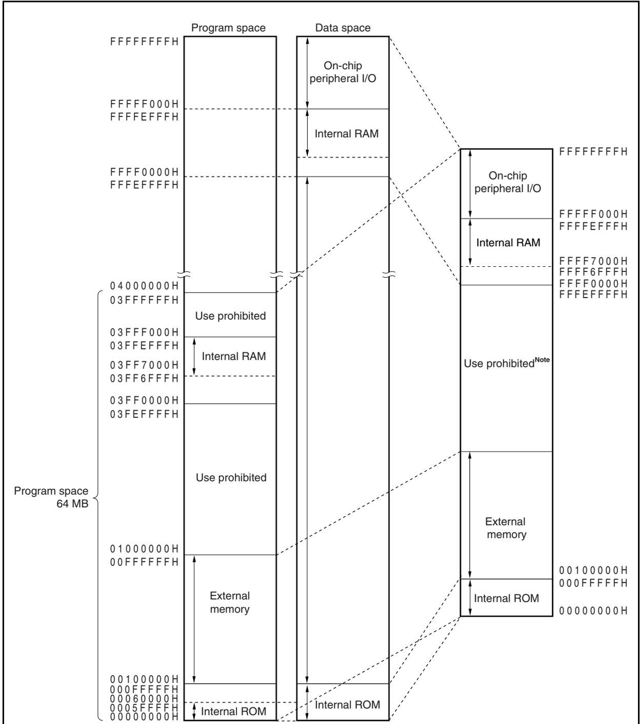
**Note** In the CAN controller version, the data space of addresses 03FEC000H to 03FEEFFFH is assigned as the programmable peripheral I/O area. Only the programmable peripheral I/O area is seen as images of 256 MB each in the 4 GB address space.
