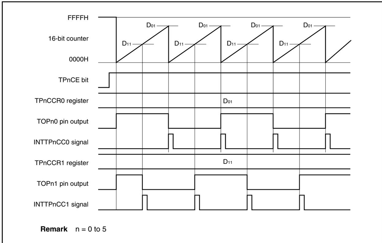
If the set value of the TPnCCR1 register is greater than the set value of the TPnCCR0 register, the count value of the 16-bit counter does not match the value of the TPnCCR1 register. Consequently, the INTTPnCC1 signal is not generated, nor is the output of the TOPn1 pin changed. When the TPnCCR1 register is not used, it is recommended to set its value to FFFFH.
