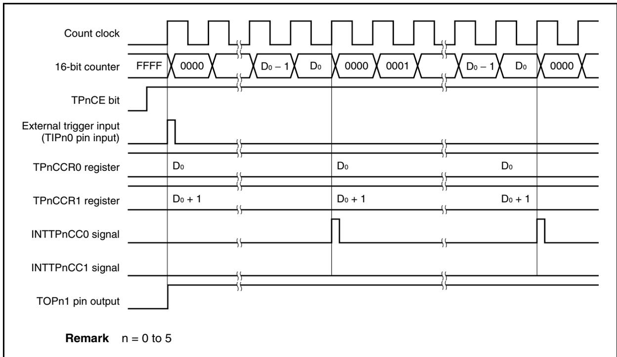
**(c) Conflict between trigger detection and match with CCR1 buffer register**
