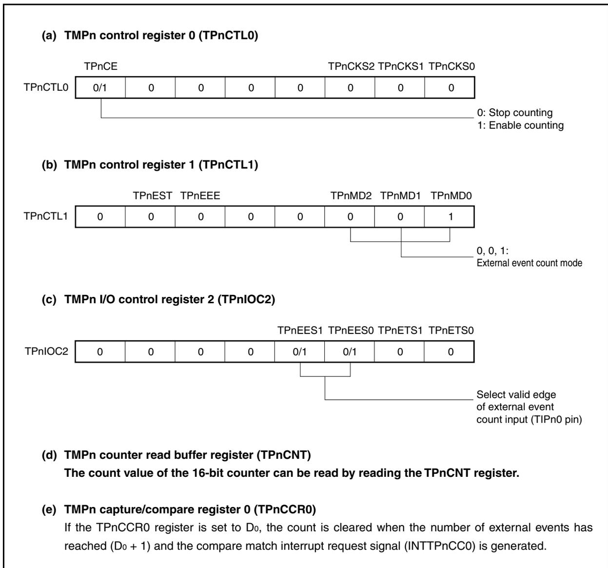
**Figure 7-15. Register Setting for Operation in External Event Count Mode (2/2)****(f) TMPn capture/compare register 1 (TPnCCR1)**
