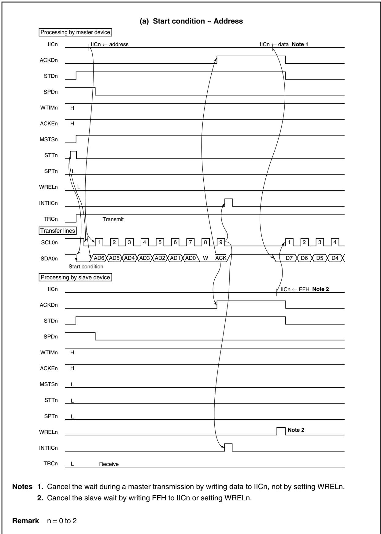
**Figure 17-20. Example of Master to Slave Communication
