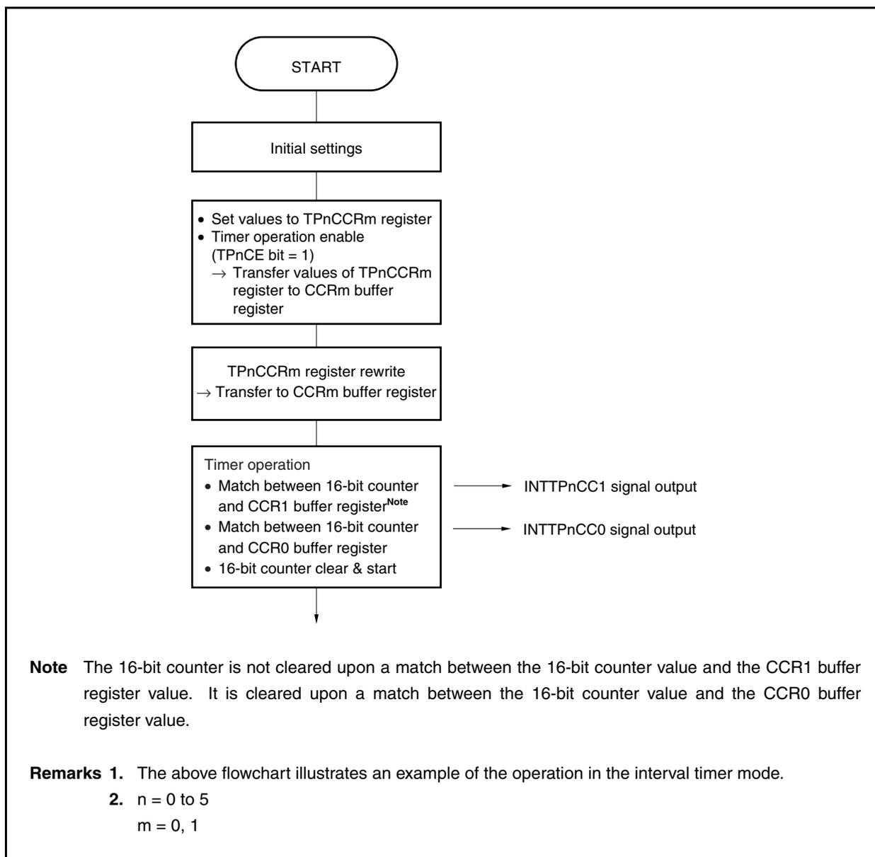
Figure 7-3. Timing of Anytime Write
