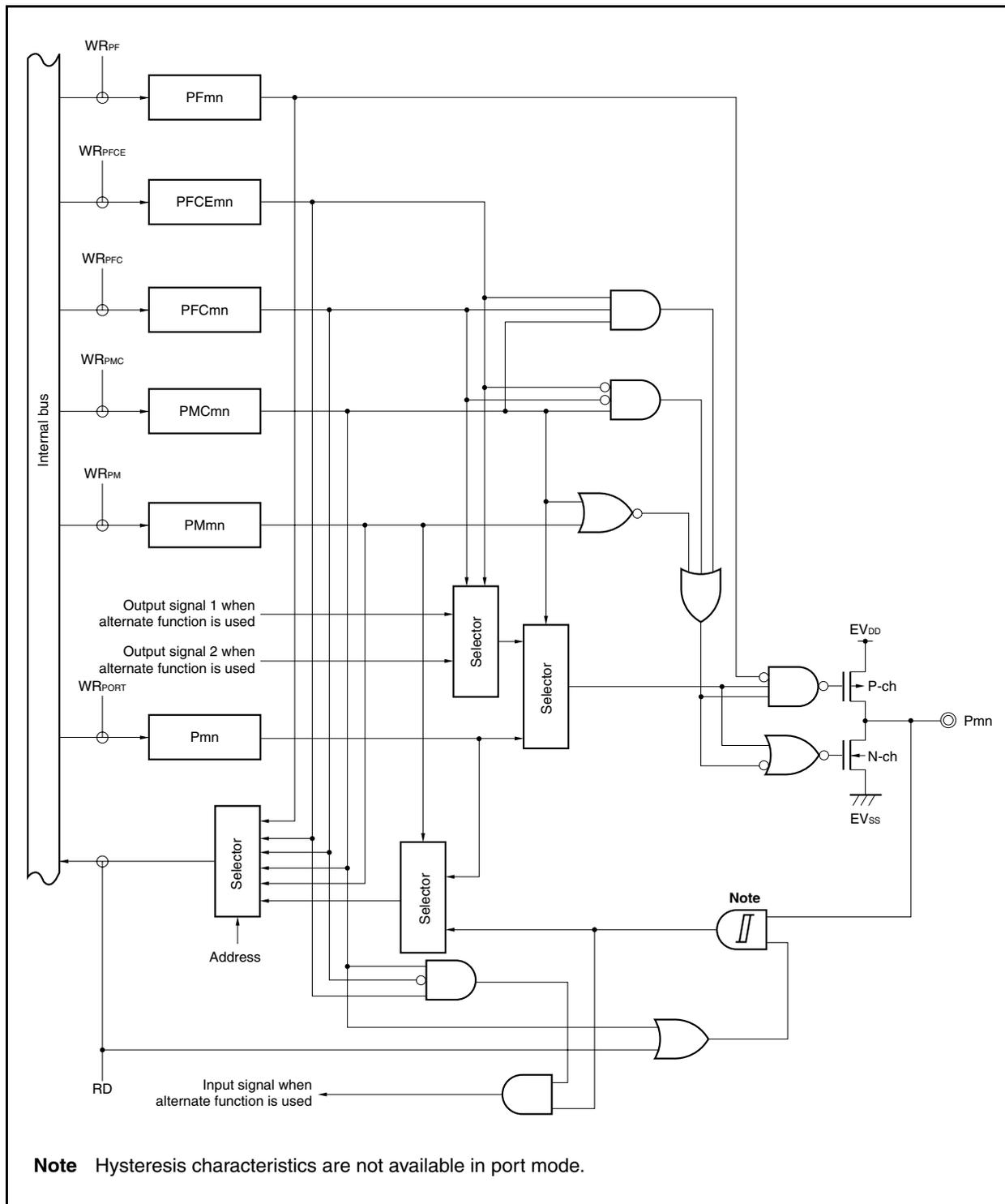
Figure 4-30. Block Diagram of Type U-14
