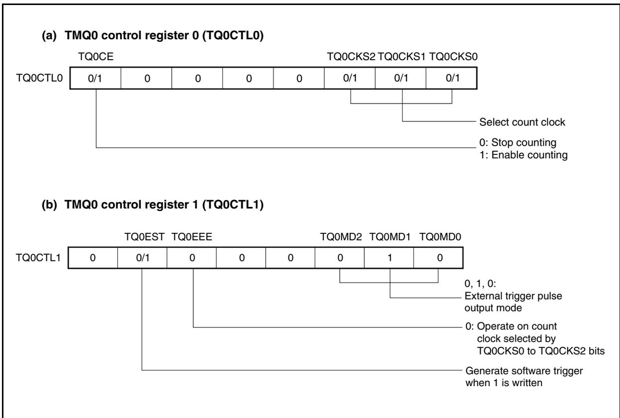
Figure 8-22. Setting of Registers in External Trigger Pulse Output Mode (2/3)
