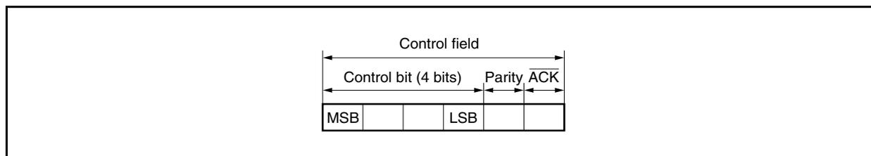
**Table 18-5. Acknowledge Signal Output Condition of Control Field**
