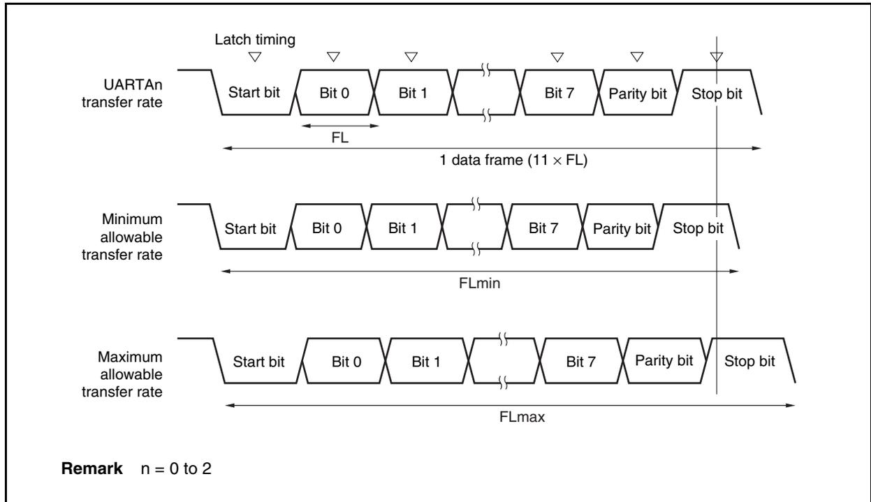
As shown in Figure 15-16, the receive data latch timing is determined by the counter set using the UAnCTL2 register following start bit detection. The transmit data can be normally received if up to the last data (stop bit) can be received in time for this latch timing.
