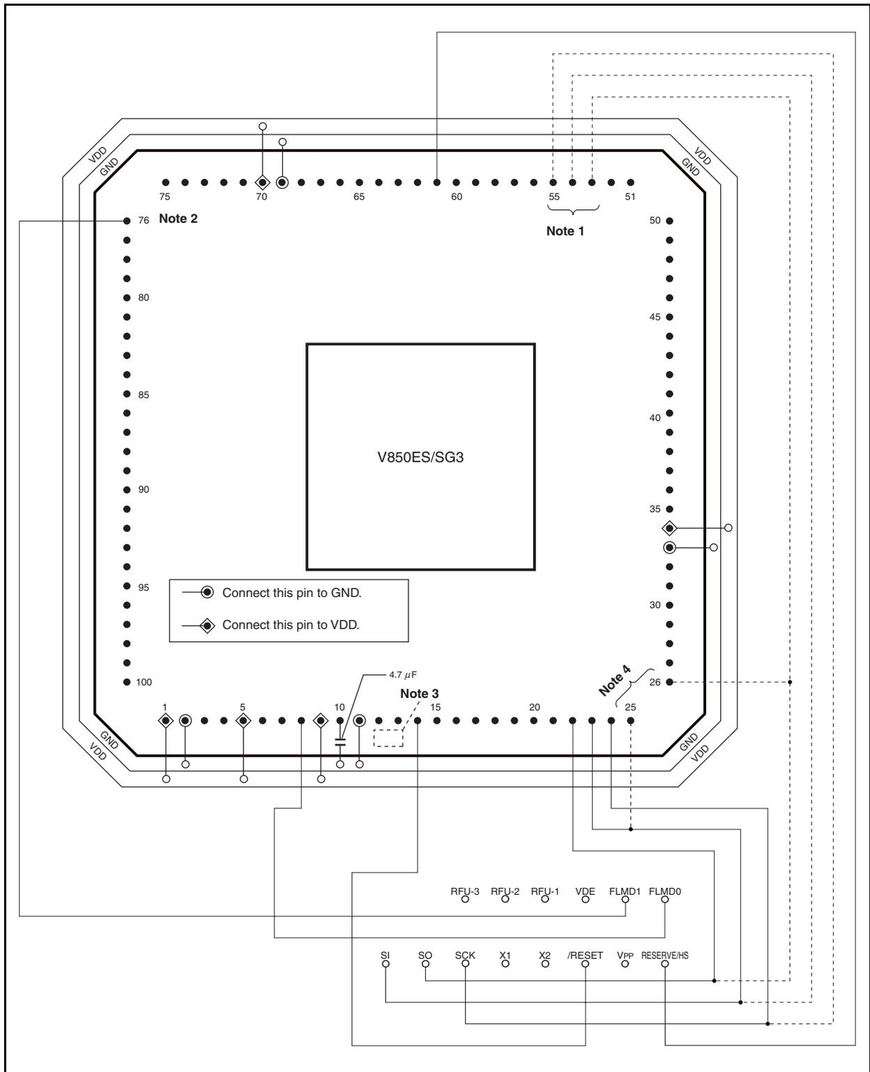
**Figure 30-6. Wiring Example of V850ES/SG3 Flash Writing Adapter (FA-100GC-8EU-A)
