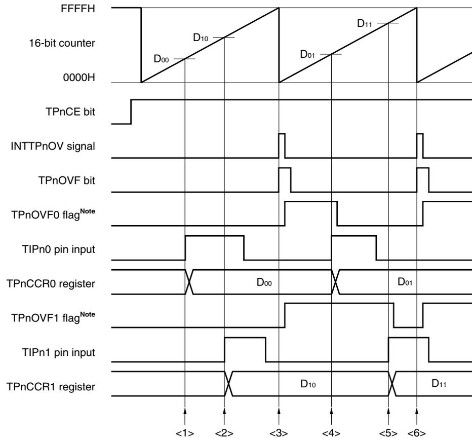
**Note** The TPnOVF0 and TPnOVF1 flags are set on the internal RAM by software.
