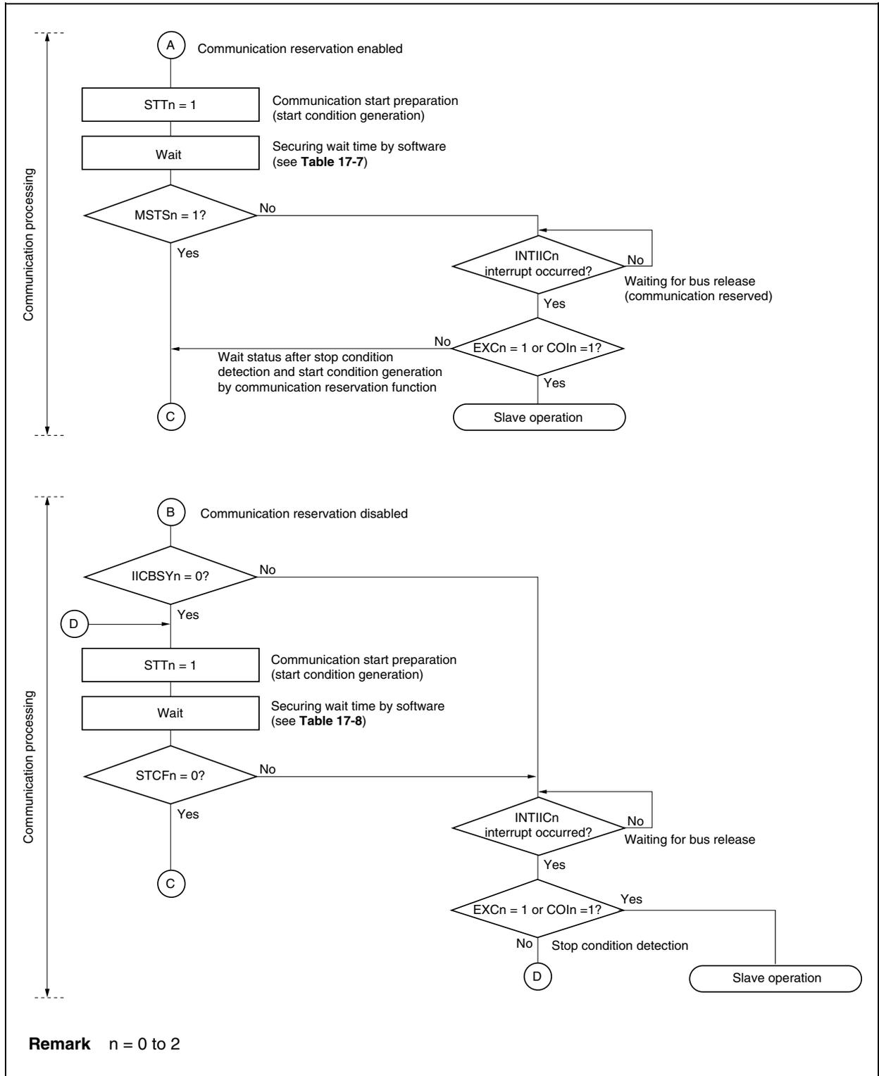
Figure 17-16. Master Operation in Multimaster System (3/3)
