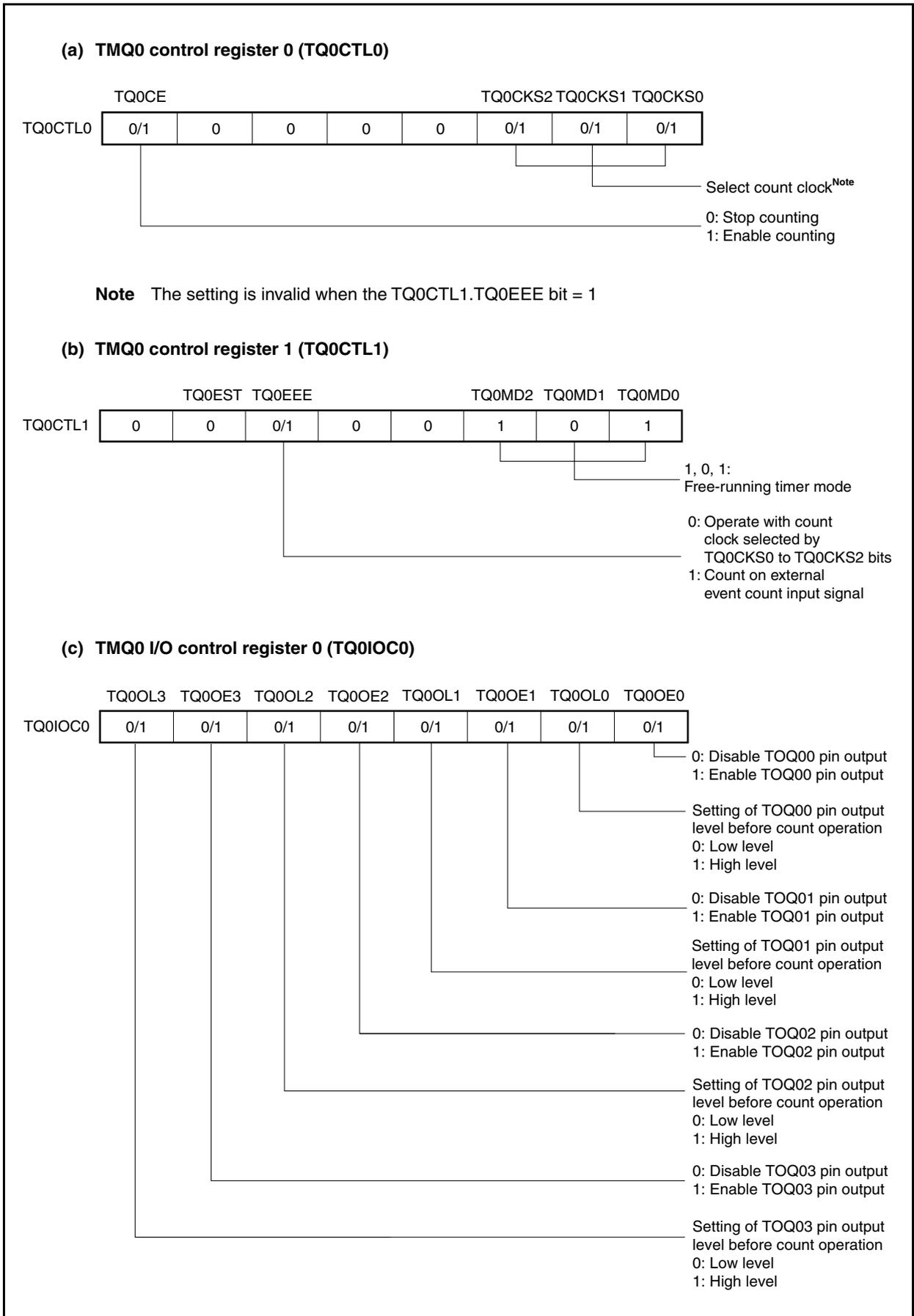
Figure 8-35. Register Setting in Free-Running Timer Mode (2/3)
