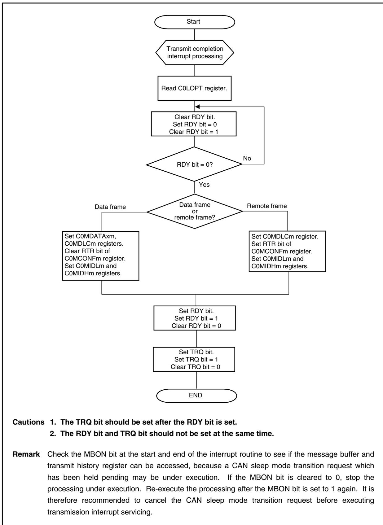
Figure 19-44. Transmission via Interrupt (Using C0TGPT Register)
