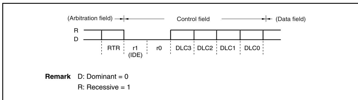
In a standard format frame, the control field's IDE bit is the same as the r1 bit.
