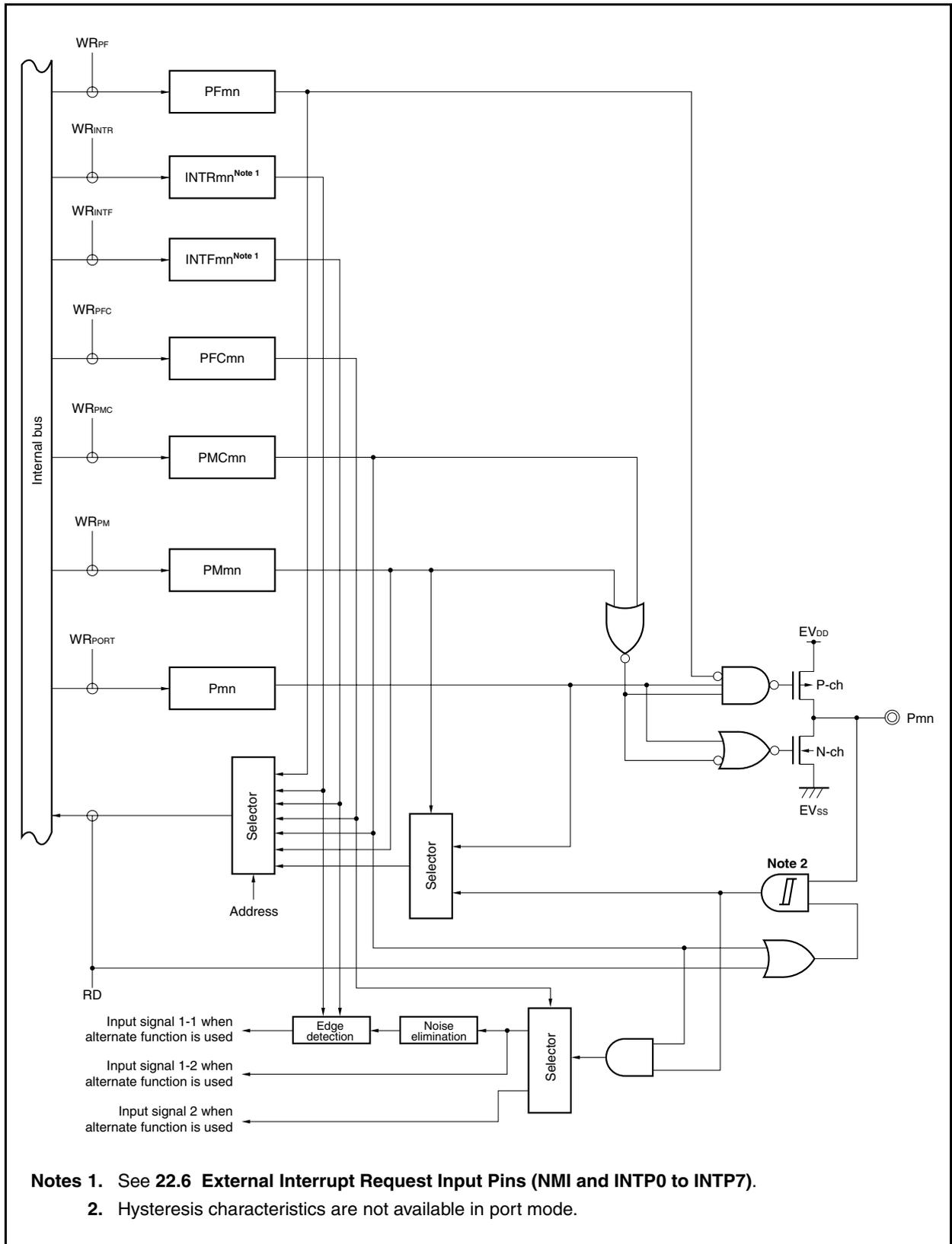
Figure 4-20. Block Diagram of Type U-1
