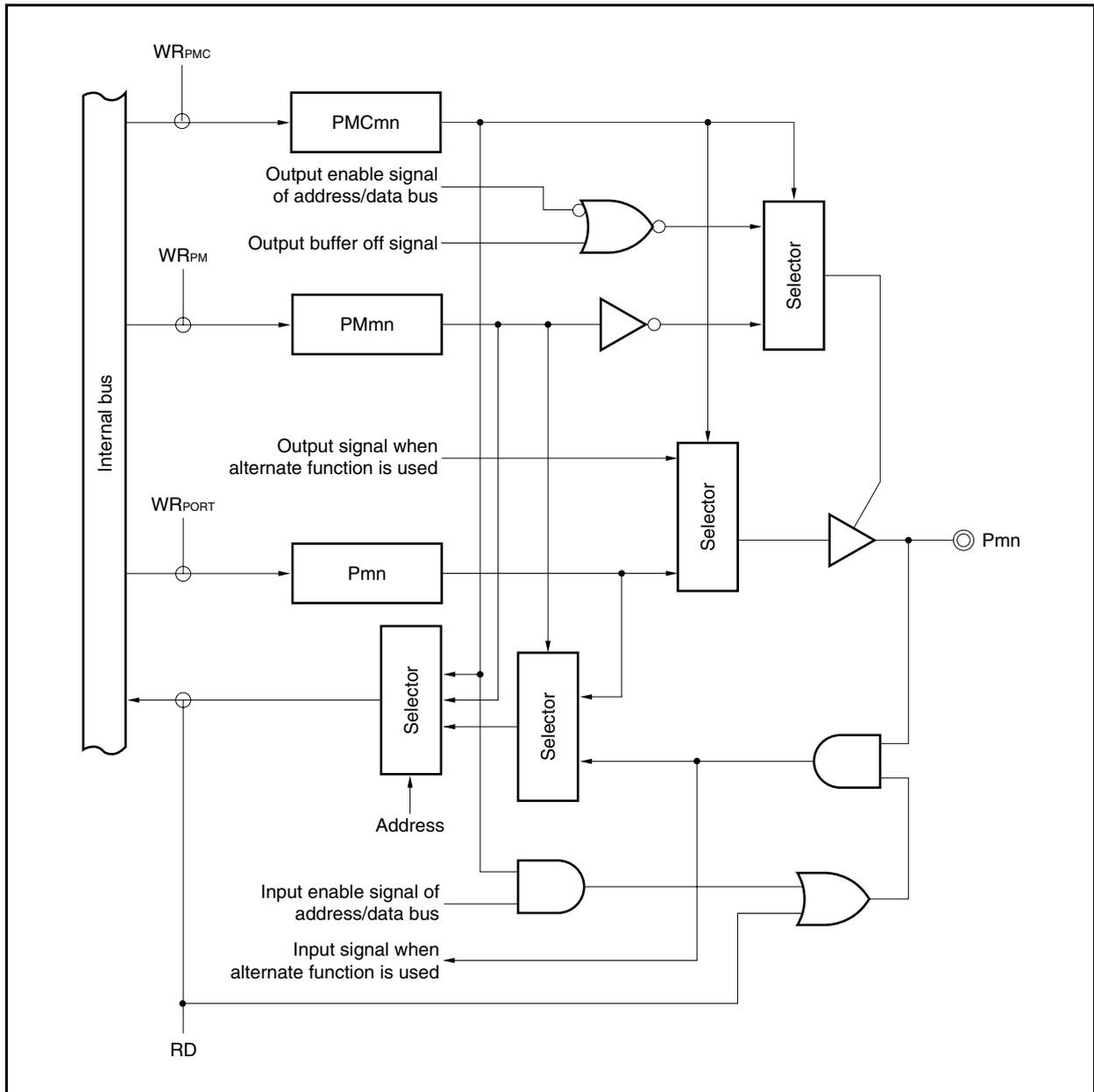
Figure 4-8. Block Diagram of Type E-3
