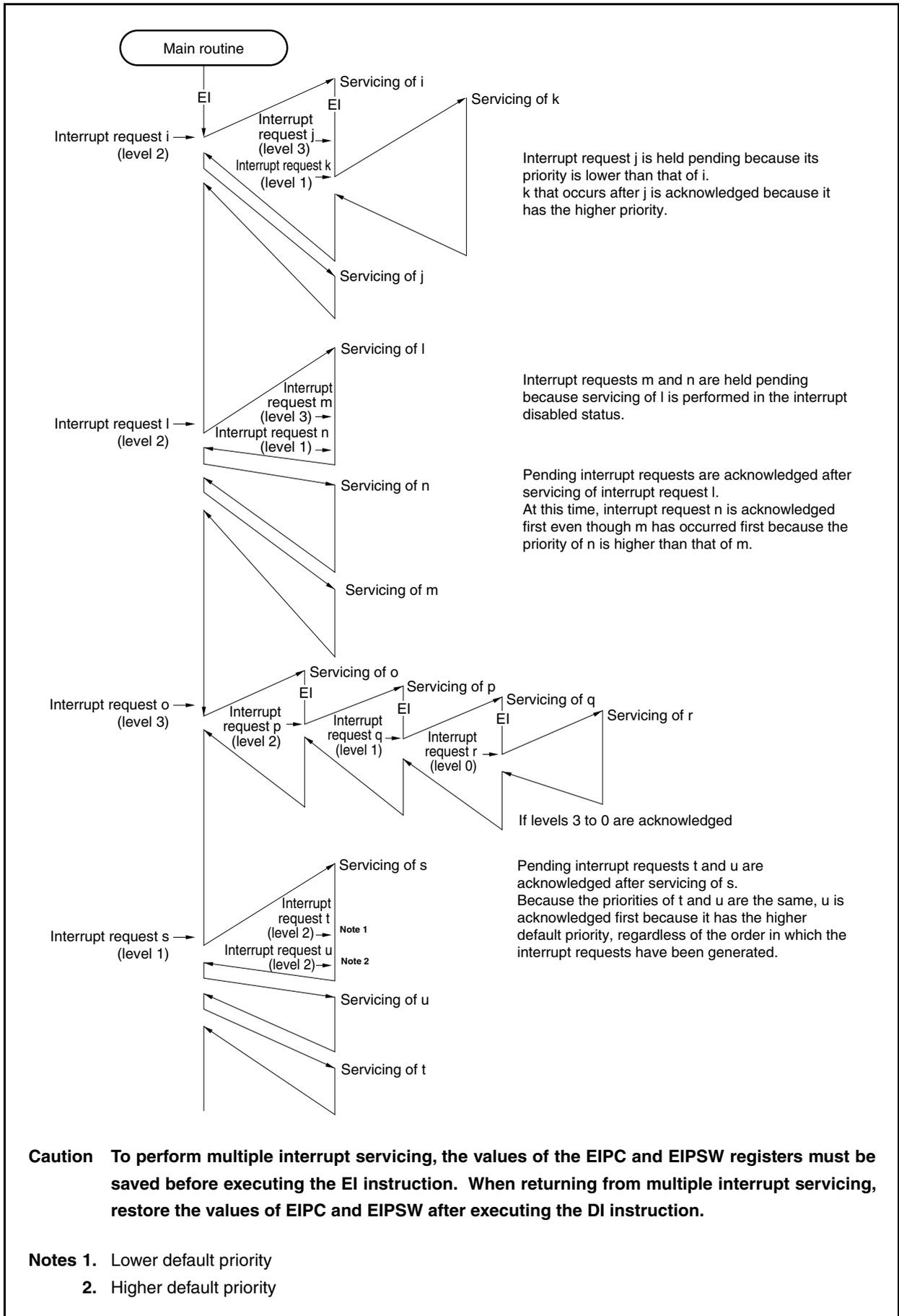
Figure 22-8. Example of Servicing Interrupt Request Signals Simultaneously Generated
