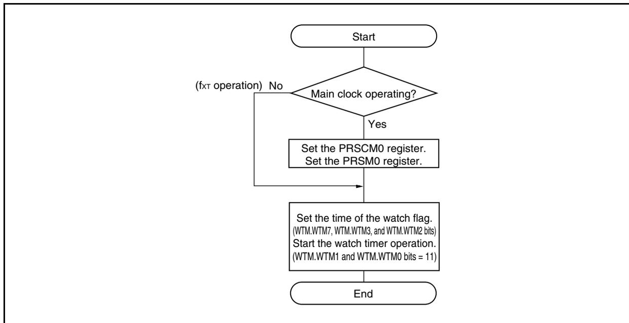
**Figure 10-3. Operation Stop Flow**
