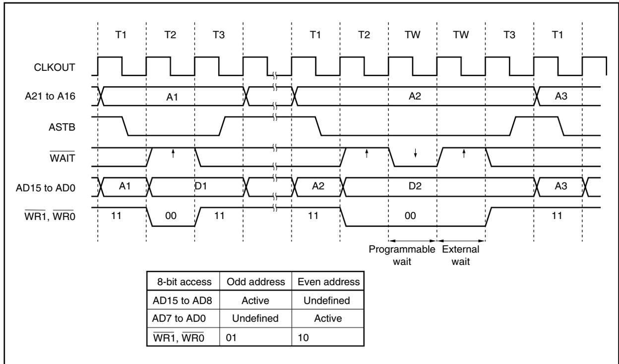
Figure 5-7. Multiplexed Bus Write Timing (Bus Size: 8 Bits)
