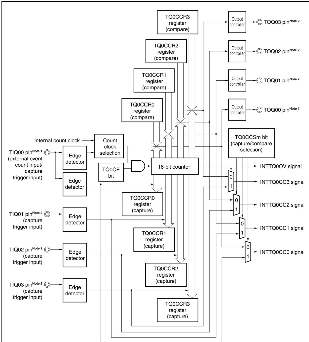
**Notes 1.** Because the external event count input pin (TIQ00), capture trigger input pin (TIQ00), and timer output pin (TOQ00) share the same alternate-function pin, two or more functions cannot be used at the same time.
