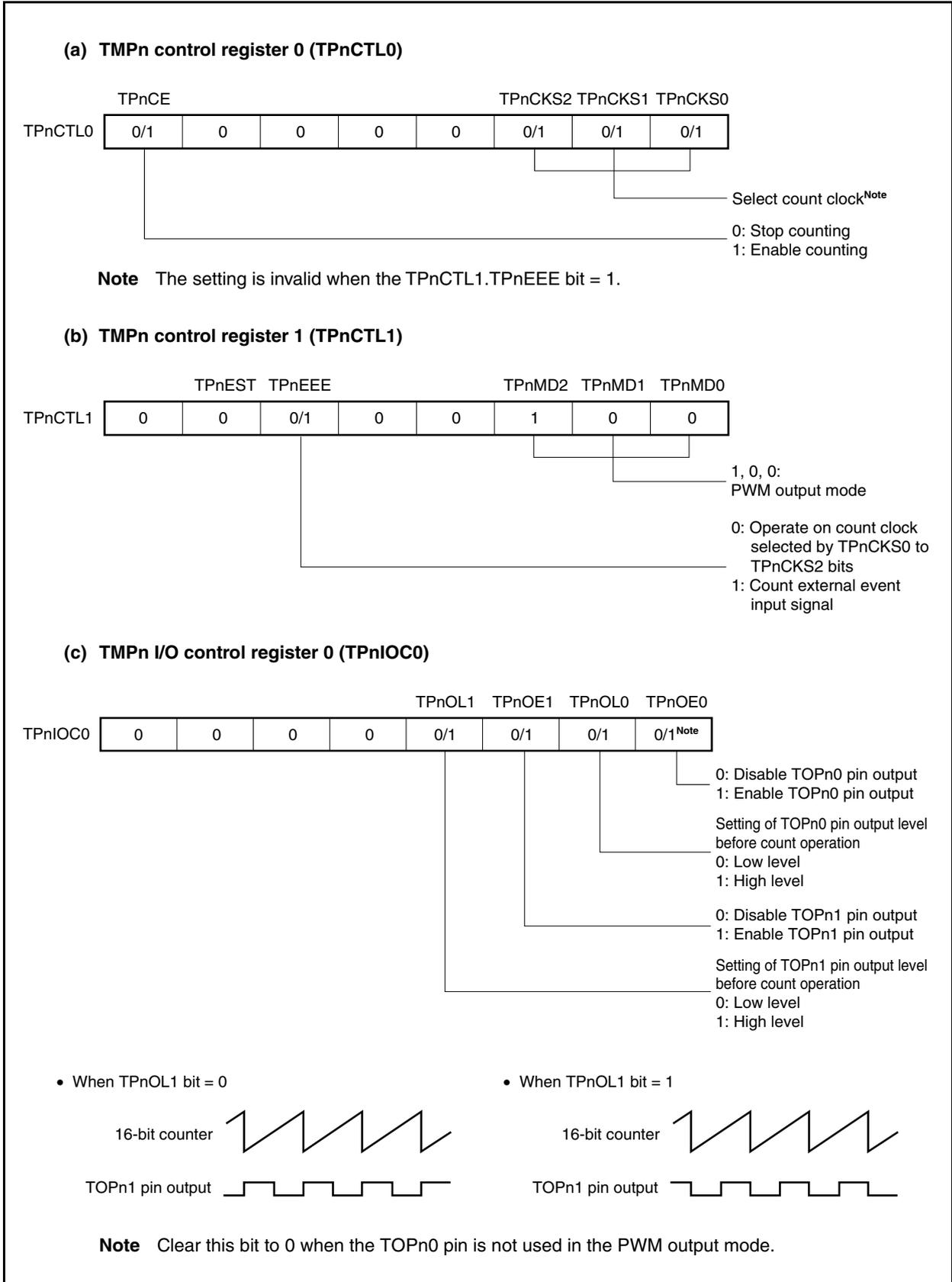
Figure 7-30. Register Setting in PWM Output Mode (2/2)
