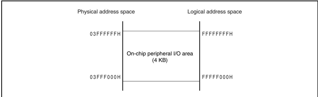
Peripheral I/O registers that have functions to specify the operation mode for and monitor the status of the on-chip peripheral I/O are mapped to the on-chip peripheral I/O area. Program cannot be fetched from this area.
