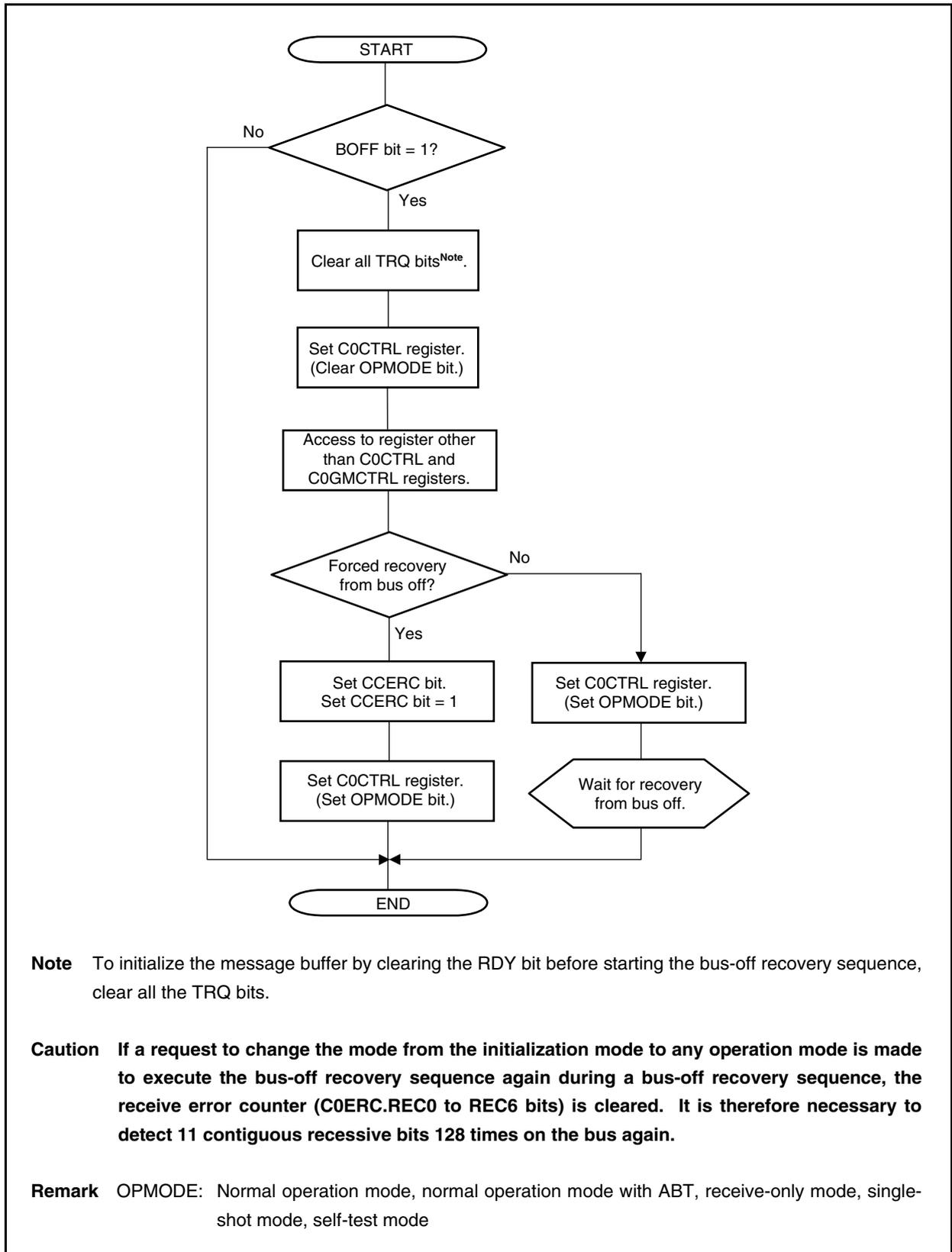
Figure 19-55. Bus-off Recovery (Normal Operation Mode with ABT)
