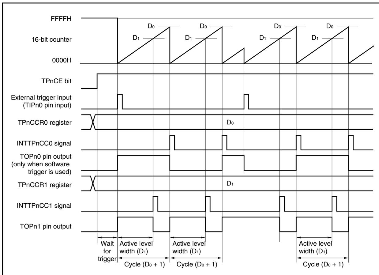
16-bit timer/event counter P waits for a trigger when the TPnCE bit is set to 1. When the trigger is generated, the 16-bit counter is cleared from FFFFH to 0000H, starts counting at the same time, and outputs a PWM waveform from the TOPn1 pin. If the trigger is generated again while the counter is operating, the counter is cleared to 0000H and restarted. (The output of the TOPn0 pin is inverted. The TOPn1 pin outputs a high-level regardless of the status (high/low) when a trigger occurs.)
