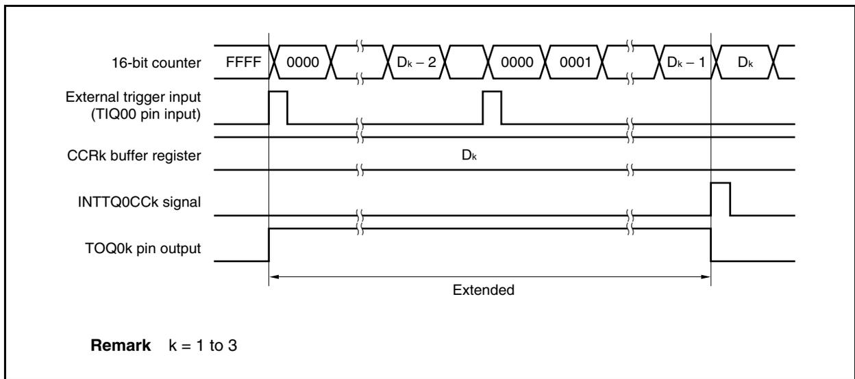
**(d) Conflict between trigger detection and match with CCR0 buffer register**
