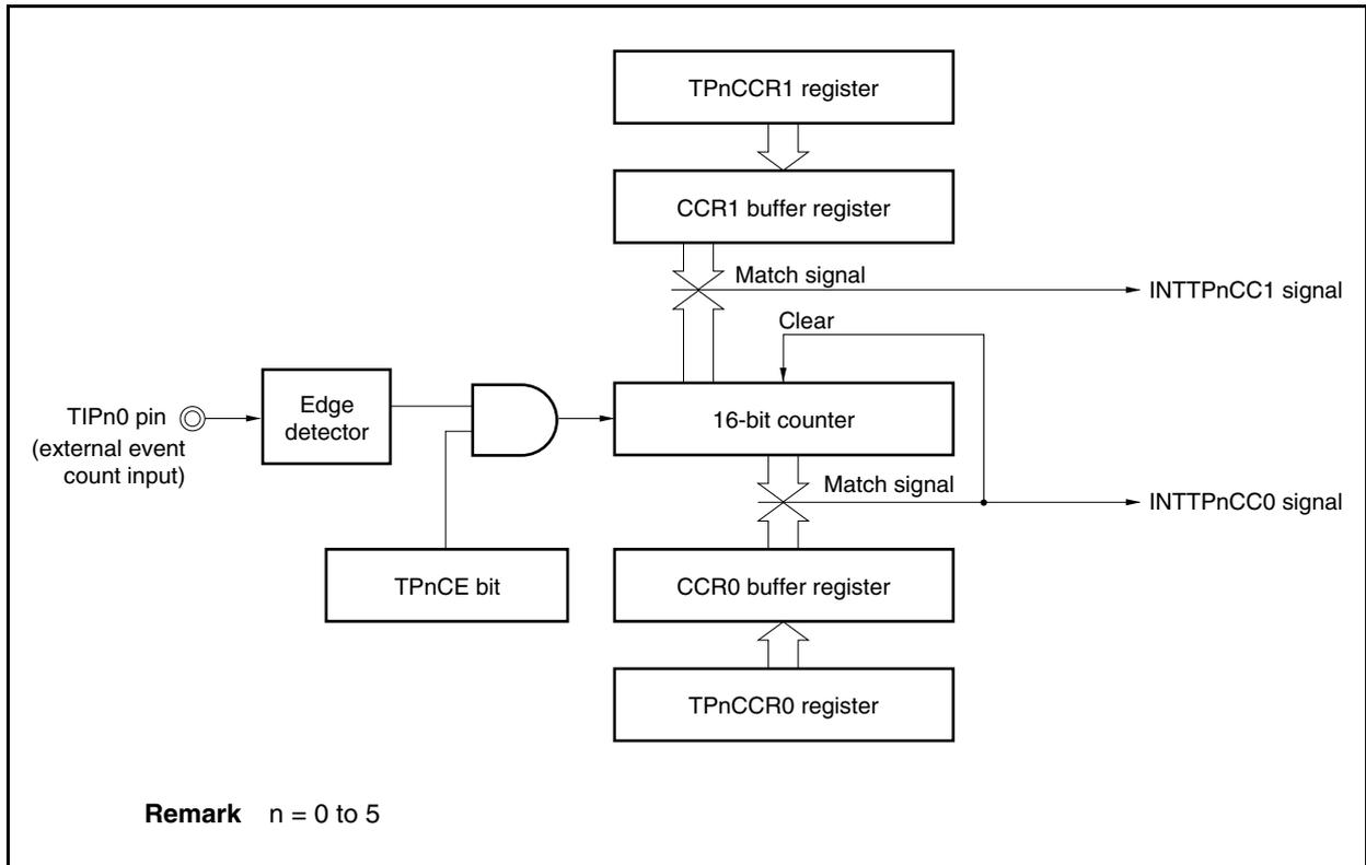
If the set value of the TPnCCR1 register is smaller than the set value of the TPnCCR0 register, the INTTPnCC1 signal is generated once per cycle.
