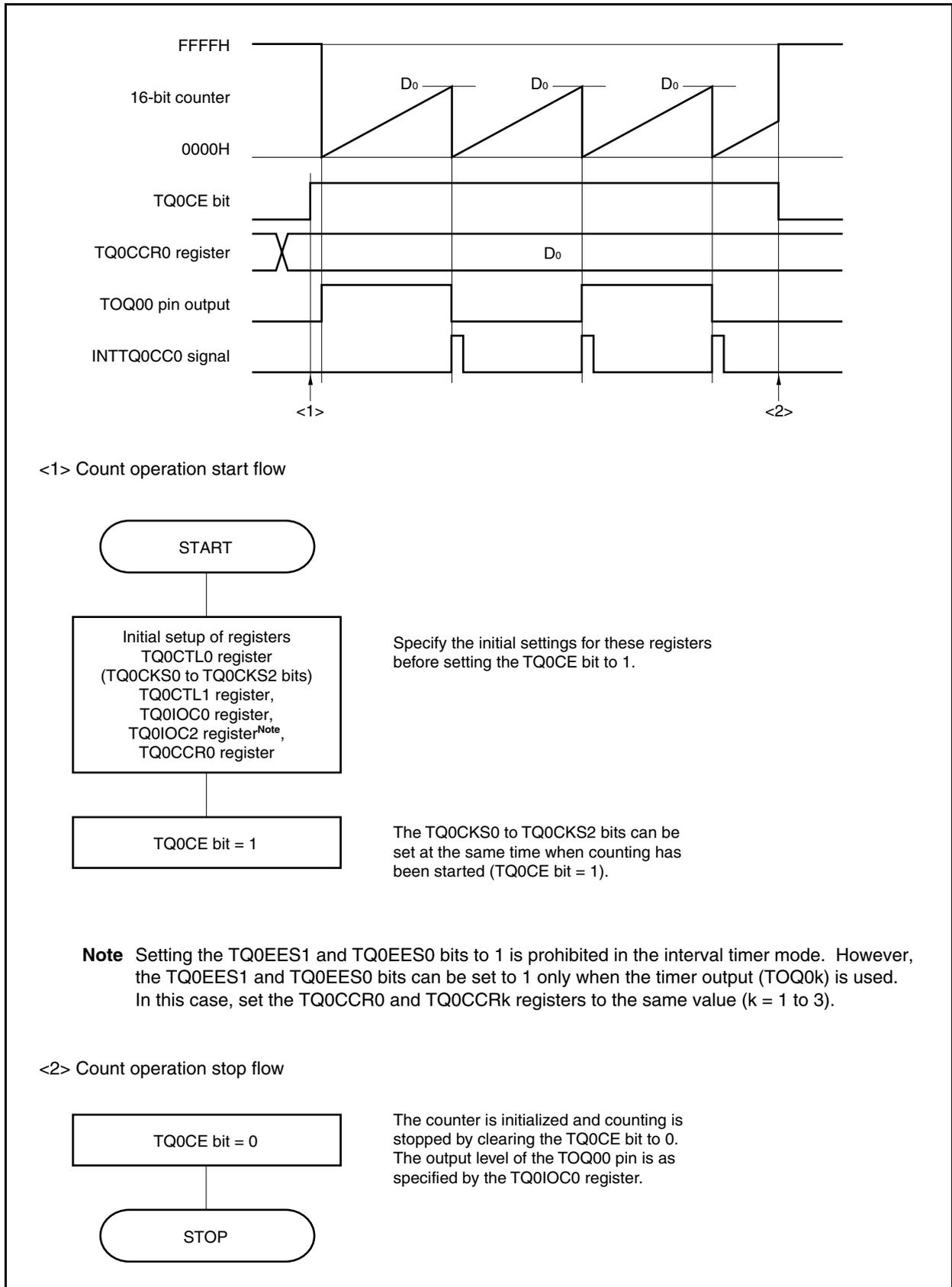
**(2) Interval timer mode operation timing****(a) Operation if TQ0CCR0 register is set to 0000H**
