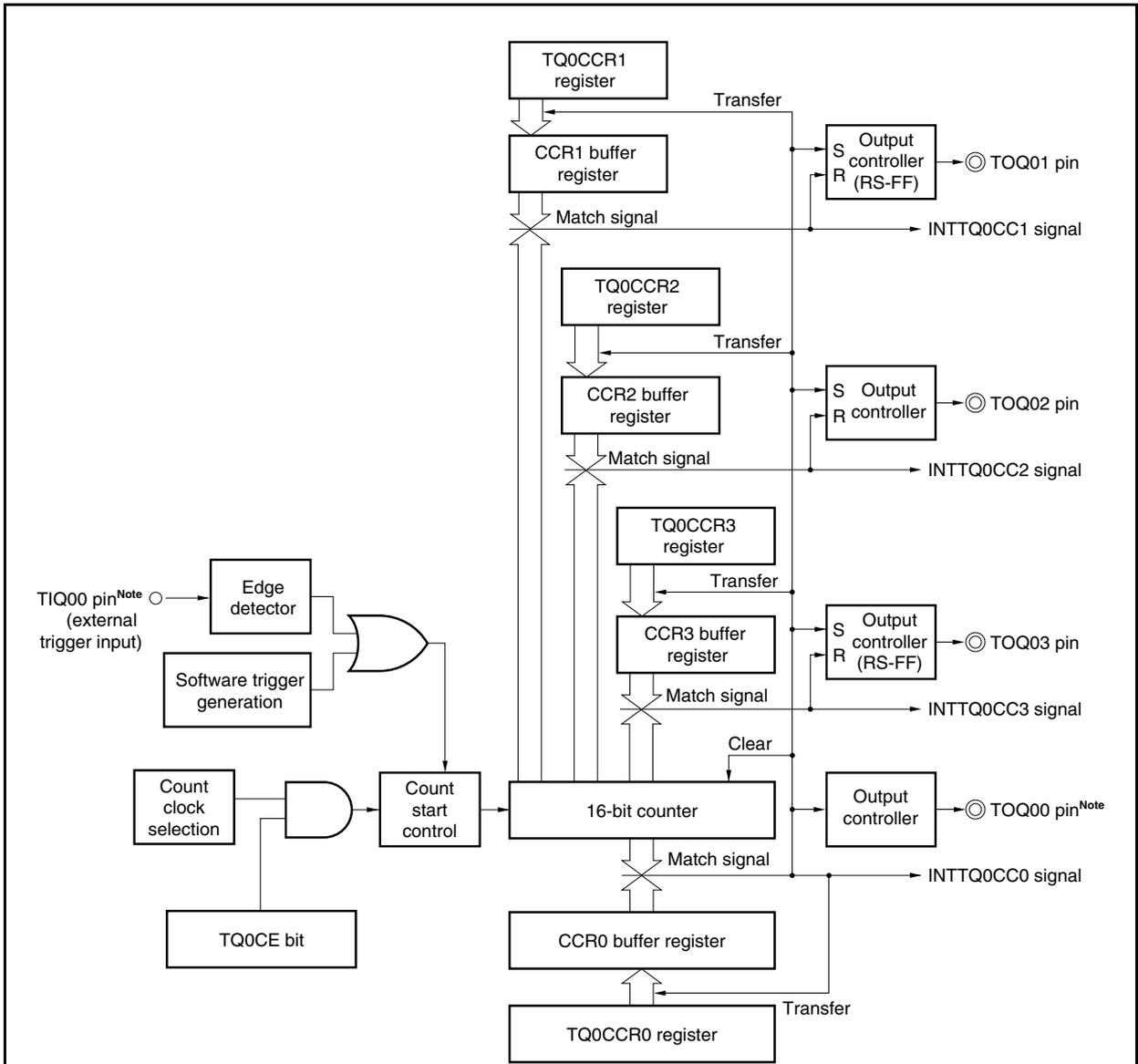
**Note** Because the external trigger input pin (TIQ00) and timer output pin (TOQ00) share the same alternate-function pin, two functions cannot be used at the same time.
