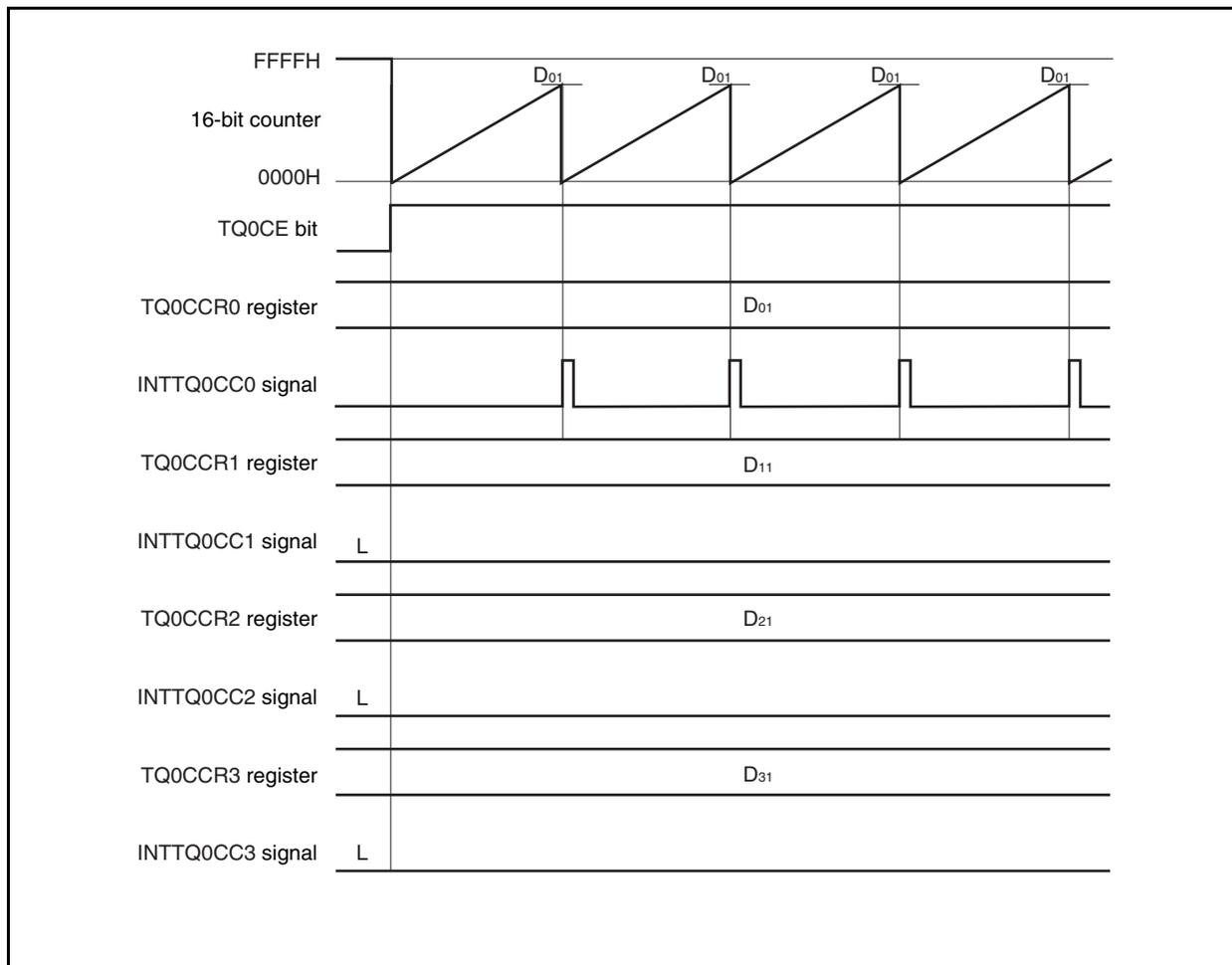
8.6.3 External trigger pulse output mode (TQ0MD2 to TQ0MD0 bits = 010)
