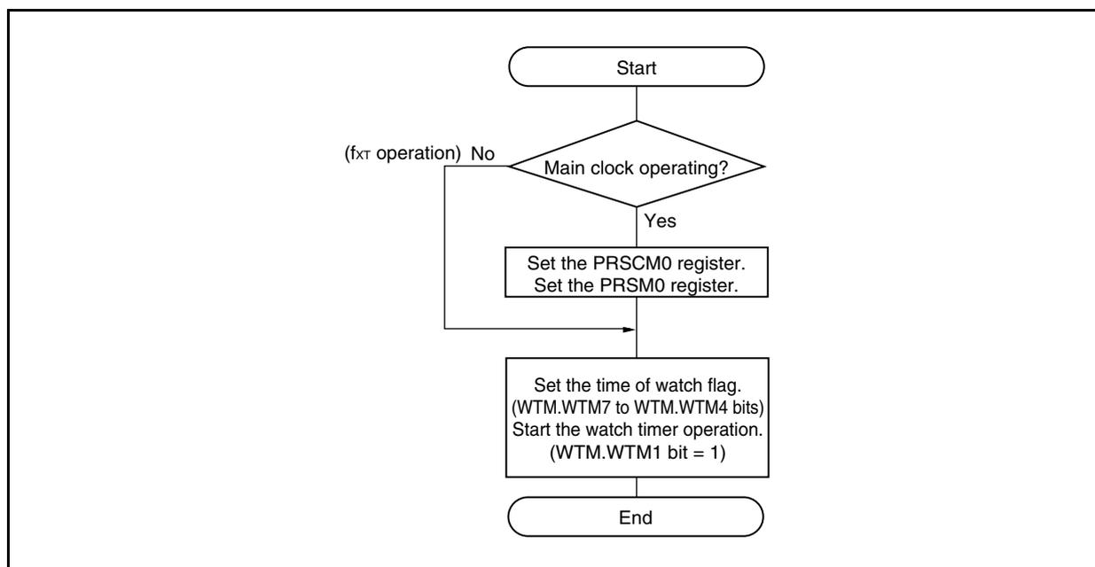
**Figure 10-5. Operation Stop Flow**
