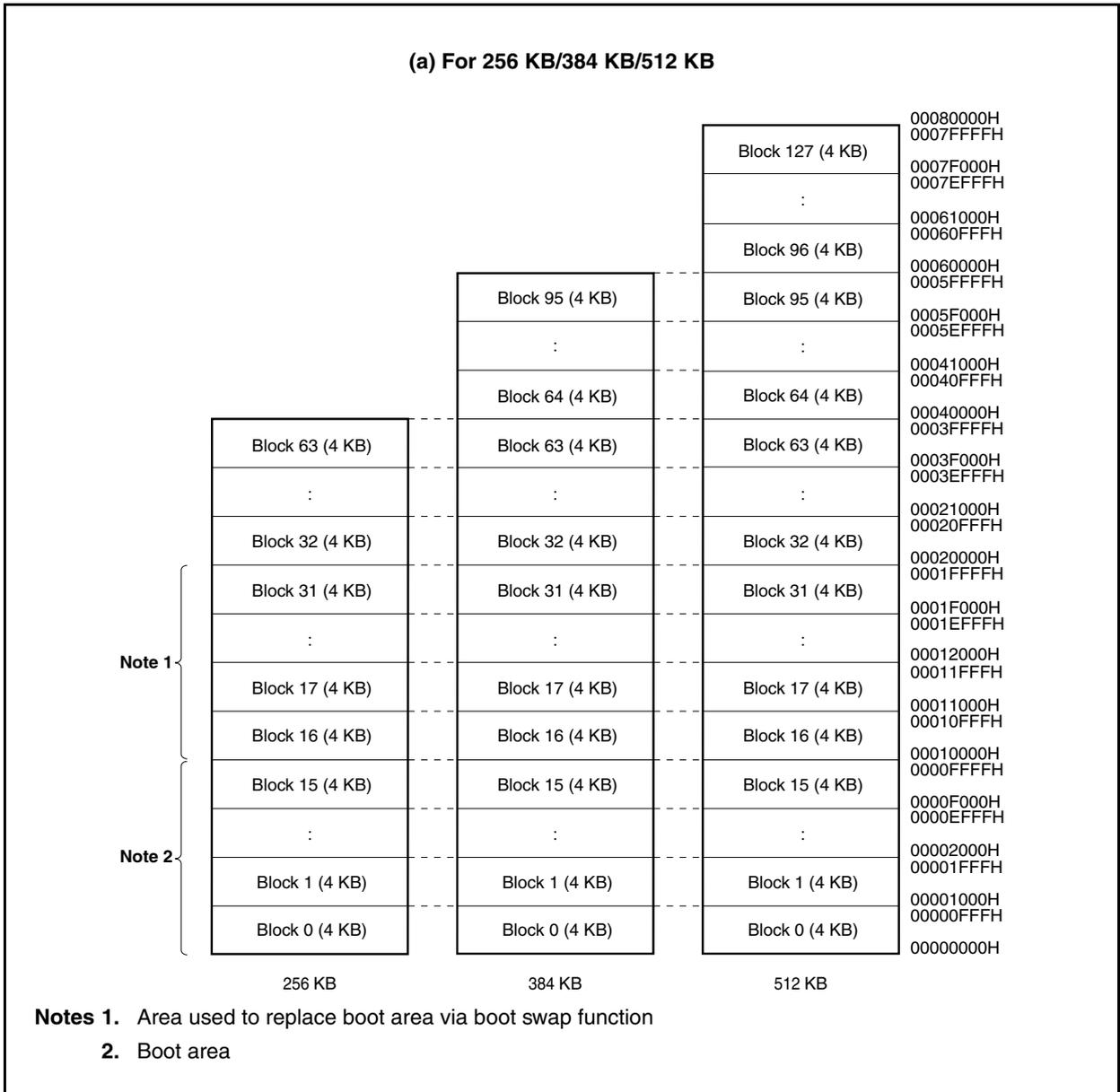
Figure 30-1. Flash Memory Mapping (2/2)
