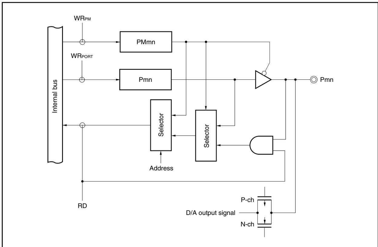
Figure 4-5. Block Diagram of Type D-1
